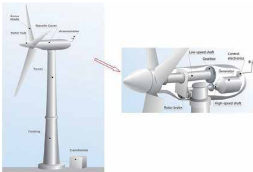
Figure 3. Schematic of a wind turbine generation system [50].
