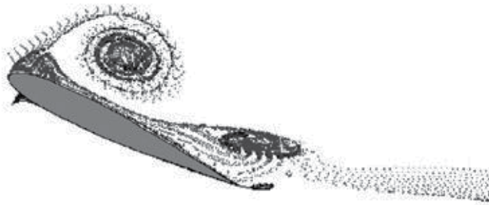
Figure 7. Aerodynamic stall mechanism- Vortex creation at the leading edge
