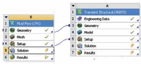
Figure 24. ANSYS workbench divergence flow-chart
