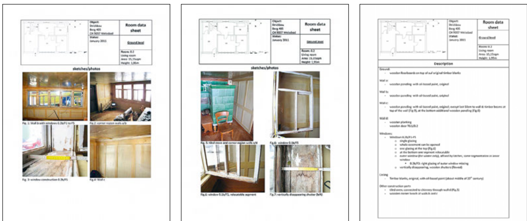
Fig. 3.2: Typical ‘as-built’ survey of one room in a ‘Raumbuch’, as practiced in Case Study 8
