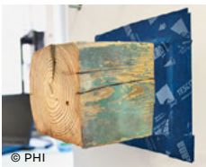
Fig. 5.10: Attempt to seal the joint of a beam with a wood panel using airtight adhesive tape
