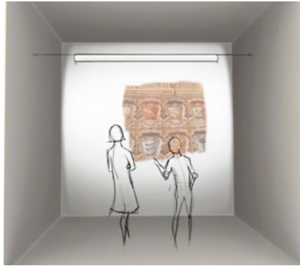
Fig. 5.52: Non-invasive installation on a cable, illuminating a precise rectangle
