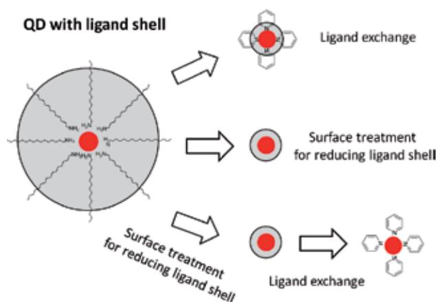
Fig. 4. Schematic illustration of two post-synthetic QD treatment strategies to enhance the PCEs in hybrid solar cells: ligand exchange (up) and reduction of the ligand surface of QDs by applying a washing procedure (middle). A combination of the two approaches might be beneficial for further enhancing the performance of hybrid solar cells (down).
