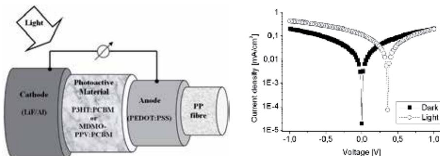
Fig. 14. Schematic drawing of a photovoltaic fiber and I-V curves of P3HT:PCBM-based photovoltaic fibers, lighting through the cathode direction. The final, definitive version of this paper has been published in < Textile Research Journal>, 80/11/July/2010 by <<SAGE Publications Ltd.>>/<<SAGE Publications, Inc.>>, All rights reserved. ©.
