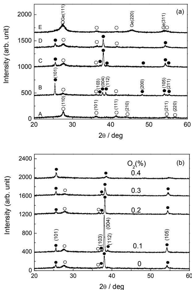
Fig. 2.1. (a) XRD patterns of Ge/TiO<sub>2</sub> composite films versus Ge concentrations. (●) indicates anatase structure, and (○), rutile structure. (b) Same patterns versus additional oxygen ratio in argon. (●) indicates anatase structure, and (○), rutile structure (b) (after Abe et al., 2008b).
