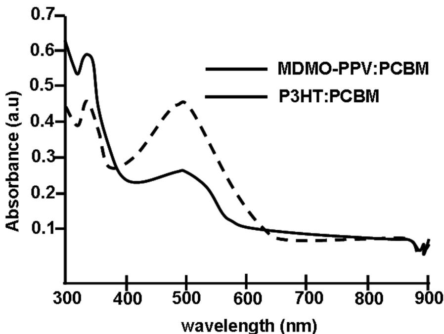
Fig. 10. Absorption spectra<sup>57</sup> for solutions of P3HTPCBM and MDMO-PPV-PCBM (with permission)
