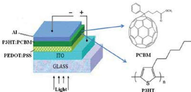
Fig. 8. Layer structure of the polymer solar cells investigated in this work.
