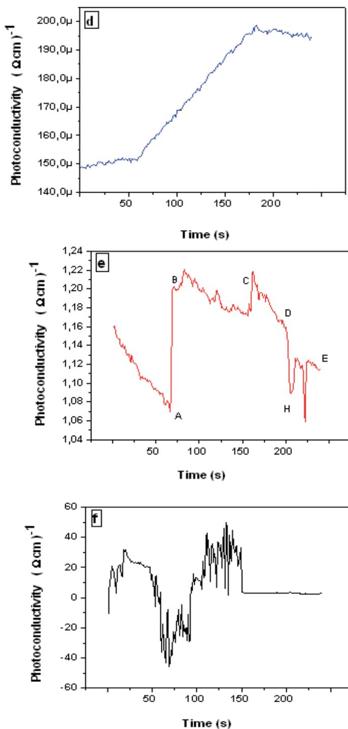
Fig. 7. Photoconductivity spectra versus time of ZnO/FTO (d), AZO/FTO (e), IZO/FTO (f).
