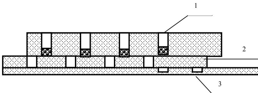
Fig. 4.3. Slide boat for growth from finite melt: 1, boat body with container for melts; 2, slider with container for finite melts; 3, slider for the substrates.
