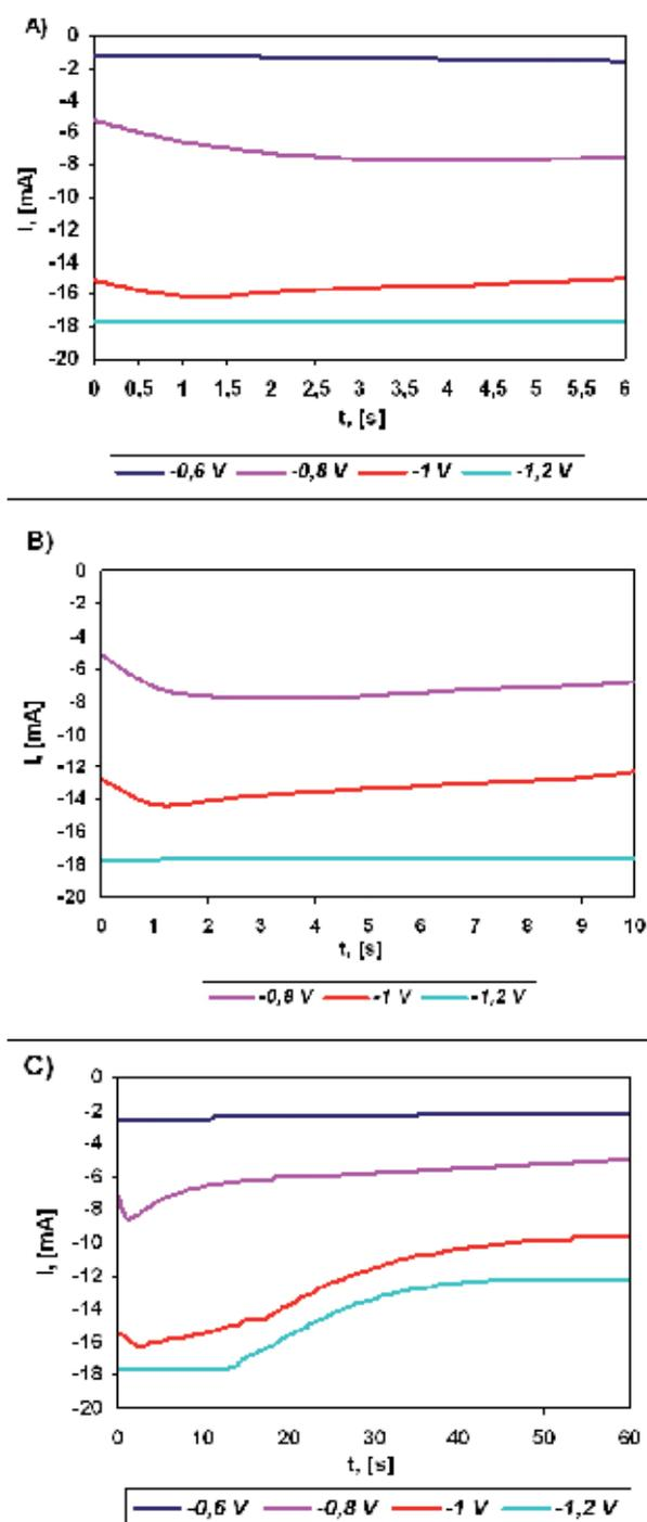
Fig. 6. Current density vs. time curves for electrodeposition of  $\text{Cu}_2\text{O}$  thin film on titanium electrode (electrodeposition time: (A) 6 s, (B) 10 s and (C) 60 s;  $t = 25^\circ\text{C}$ , pH 9.22)
