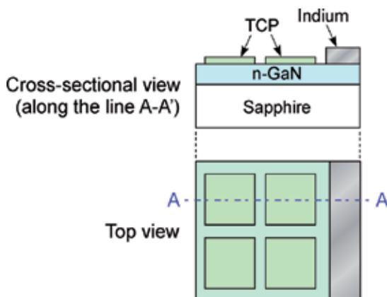
Fig. 2. Schematic of TCP/epi.-GaN sample.
