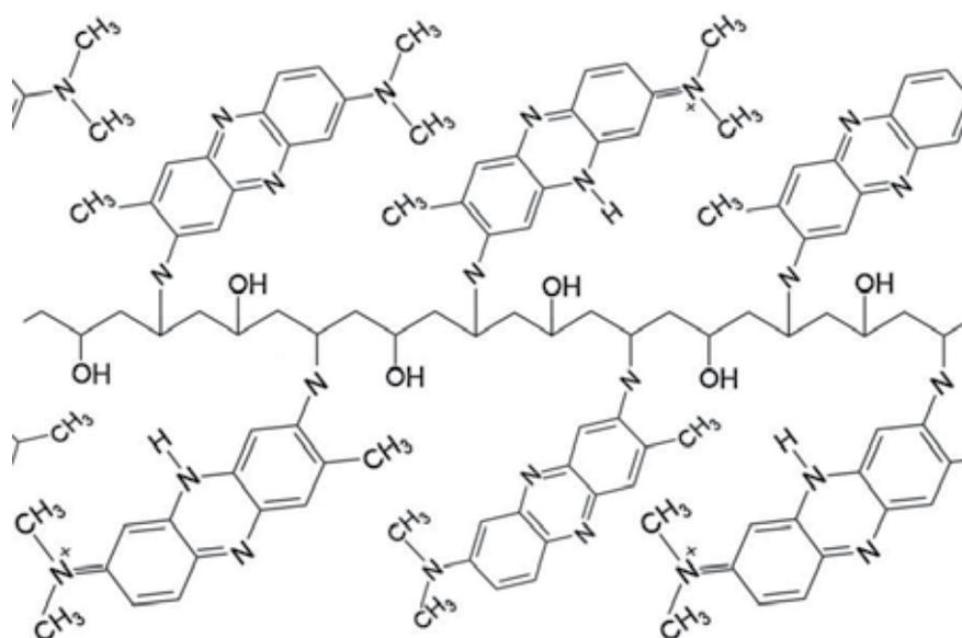
Fig. 2. Schematic structure of polyvinyl-NR that is produced by covalent bond between amine of NR and alcohol of polyvinyl alcohol. The polyvinyl-NR can bind physically to graphite cathode surface.
