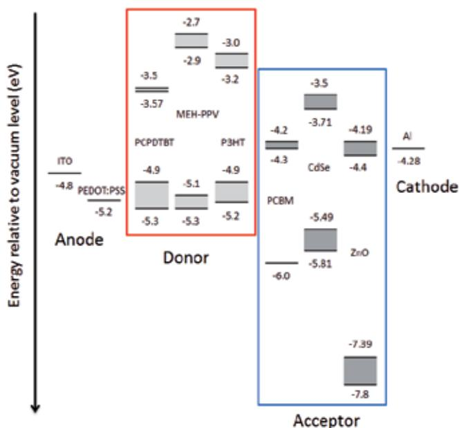
Fig. 3. Energy levels (in eV) of commonly used conjugated polymers as electron donors and NCs as electron acceptors in bulk-heterojunction hybrid solar cells.
