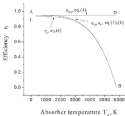
Fig. 8. Comparison of the efficiency  $\mu_{OS}\mu_U$  of combinations of reversible working and irreversible non-working processes (the AB line) with the efficiency  $\mu_{OS}$  of a reversible Carnot working process (the AD line) and the efficiency  $\mu_L$  of reversible non-Carnot working processes (the LB line). Lines AD и AB coincide at  $T_A=0$  K.
