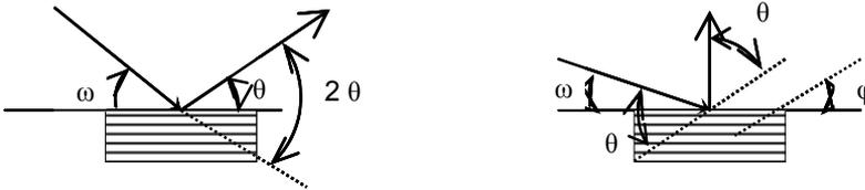
Fig. 3.3. Symmetric and asymmetric reflections from crystal surface
