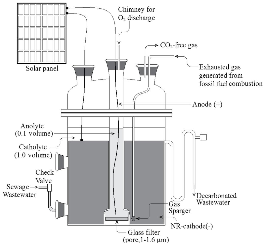
Fig. 9. Schematic diagram of the cylinder-type electrochemical bioreactor equipped with a built-in anode compartment for the cultivation of CO<sub>2</sub>-fixing bacteria. The glass filter septum equipped at the bottom end of the anode compartment functions as redox separator between anode and cathode compartment and micropore for transfer of catholyte to anode compartment.
