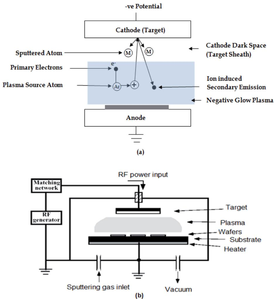
Fig. 1. Schematic Diagrams of (a) DC sputtering and (b) RF sputtering (Ohring, 2002)
