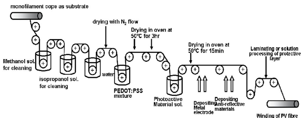
Fig. 9. Manufacturing process of Photovoltaic fibre as suggested by Bedeloglu et al.<sup>21</sup>
