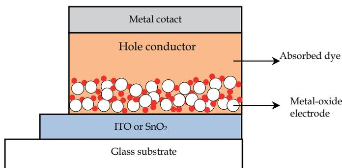
Fig. 3. Schematic of solid state dye-sensitized SC
