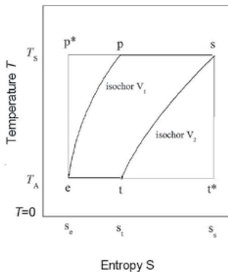
Fig. 4. Entropy diagram showing some thermodynamic cycles for conversion of solar heat into work in cavity 2 with the participation of a black body. Isotherms represent the absorption and emission of radiant energy. Lines  $pe$ ,  $p^*e$  correspond to the cooling of radiation in the black body. Line  $st$  indicates the temperature and entropy of radiation in cavity.
