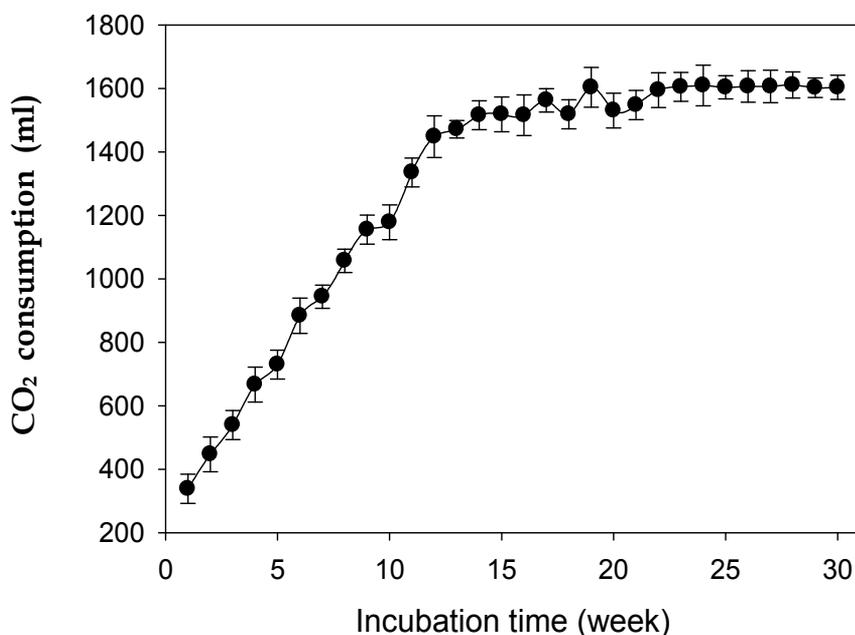
Fig. 11. Weekly consumption of CO<sub>2</sub> in the electrochemical bioreactor from the initial incubation time to 30 weeks. CO<sub>2</sub> consumption was analyzed weekly and the gas reservoir was refilled with 50±1% of CO<sub>2</sub> to N<sub>2</sub> at 4-week intervals.
