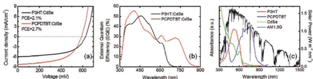
Fig. 7. (a) J-V characteristics of the best solar cells fabricated from blends of P3HT:CdSe and PCPDTBT:CdSe with a PCEs of 2.1% and 2.7% respectively. (b) EQE spectra of the P3HT:CdSe and PCPDTBT:CdSe devices (c) Absorption spectra of CdSe QDs, P3HT, PCPDTBT in thin films, in comparison with the AM1.5G solar emission spectrum.
