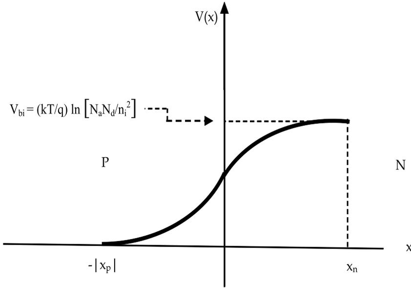
Fig. 2. Potential  $V$  as a function of  $x$  across the depletion region. Note (a) the two branches of  $V$  across both sides of the junction's boundary ( $x = 0$ ) in accordance with (4) and (5) (b) the built-in voltage  $V_{bi}$  at the right edge of the junction [1, 2, 3]. Note also that built-in voltage is normally computed as shown in the inset.
