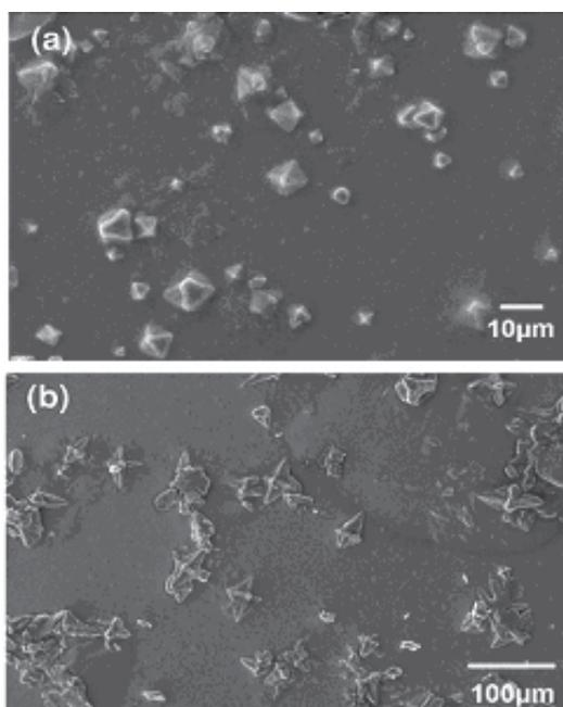
Fig. 5. The  $\text{Cu}_2\text{O}$  films synthesized under different current densities with the same deposition time (Hu et al., 2009)
