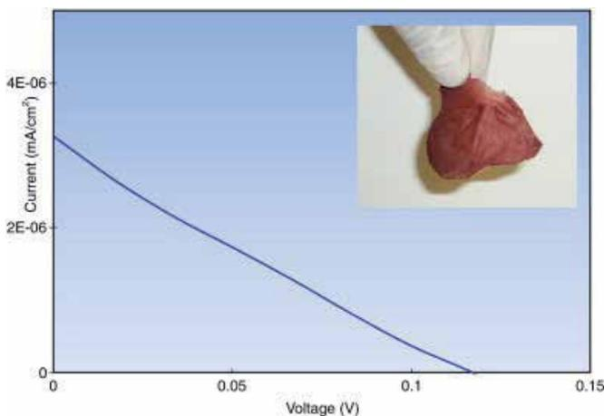
Fig. 11. Jsc-V graph of the P3HT/PCBM based solar cloth measured under 1 Sun conditions. Inset shows a picture of the solar cloth fabricated using electrospinning. Reprinted from *Materials Letters*, 64, Sundarrajan, S.; Murugan, R.; Nair, A. S. & Ramakrishna, S., 2369 -2372., Copyright (2010), with permission from Elsevier.
