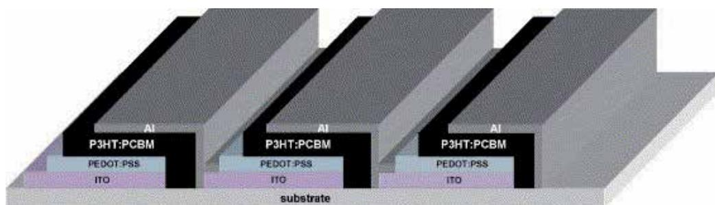
Fig. 8. Serial connection of organic solar cells. Reprinted from *Sol. Energy Mater. Sol. Cells*, 91, Lungenschmied, C.; Dennler, G.; Neugebauer, H. ; Sariciftci, N. S. ; Glatthaar, M. ; Meyer, T. & Meyer, A., Flexible, long-lived, large-area, organic solar cells, 379–384, Copyright (2007), with permission from Elsevier.
