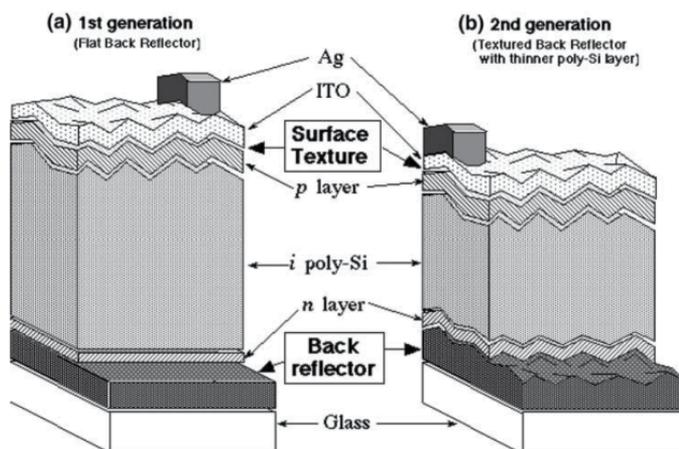
Fig. 7. Cross-sections through light-trapping  $\mu\text{c}$ -silicon SC devices: (a) first generation (flat back reflector); (b) second generation (textured back reflector, thinner polycrystalline silicon layer). Reprinted with permission from Solar Energy Vol. 77, Kenji Yamamoto et al., A high efficiency thin film silicon solar cell and module, pp. 939–949 © 2004, Elsevier.
