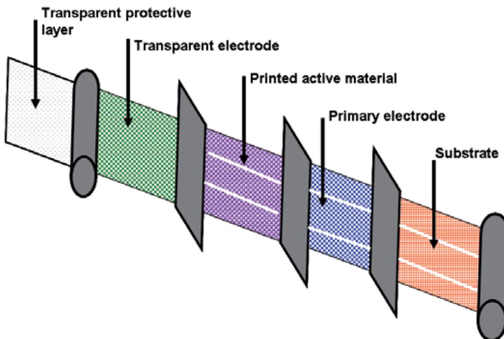
Fig. 4. Konarka's plastic photovoltaic cells by printing technology
