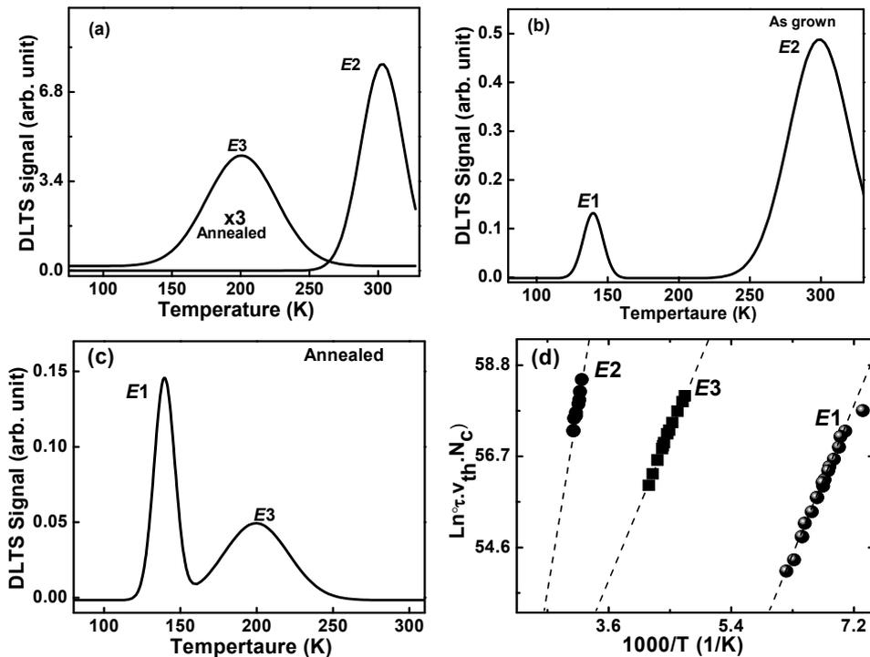
Fig. 2. DLTS spectra of (a)  $N$  free as grown and annealed GaAs, (b) as grown  $n$ -type  $GaAs_{0.998}N_{0.002}$ , (c) annealed  $n$ -type  $GaAs_{0.998}N_{0.002}$ , and (d) Arrhenius plots of DLTS spectra.
