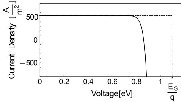
Fig. 2. The current-voltage characteristic of an SGSC with  $E_G = 1.1$  eV. The solid and dashed lines represent the  $J(V)$  function for a flat cell without concentrators, placed on Earth at a temperature of 300 K and at absolute zero (the temperature corresponding to the ultimate efficiency), respectively.
