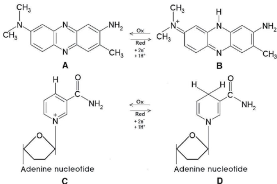
Fig. 1. Molecular structure of neutral red, which can be electrochemically oxidized (A) or reduced (B). The reduced neutral red can catalyze reduction reaction of  $\text{NAD}^+$  (C) to  $\text{NADH}$  (D) without enzyme catalysis. Ox and Red indicate oxidation and reduction, respectively.
