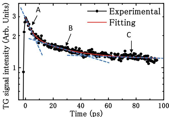
Fig. 2. TG kinetics of CdSe QDs adsorbed onto a nanostructured  $\text{TiO}_2$  film measured in air. The vertical axis is plotted on a logarithmic scale. Three decay processes A, B and C can be clearly observed (Shen et al., 2010a).
