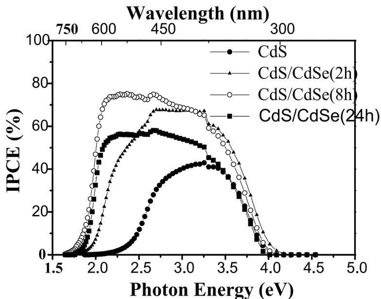
Fig. 5. IPCE spectra of nanostructured TiO<sub>2</sub> electrodes adsorbed with CdS/CdSe quantum dots for different adsorption times together with that adsorbed with CdS quantum dots only.
