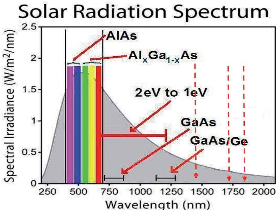
Fig. 6. Regions of the solar spectrum covered by the superlattice cell and the top cell (visible). The superlattice can be tuned at  $\sim 1$  eV. Dashed arrows indicate region of feasible absorption from the superlattice region
