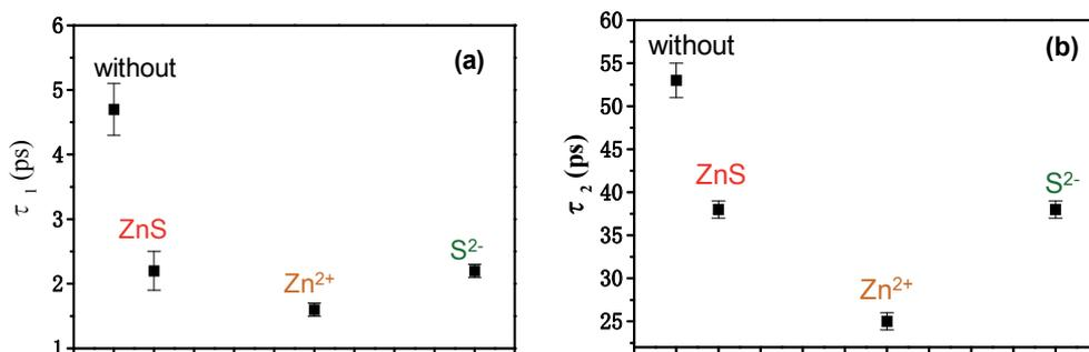
Fig. 10. Fast ( $\tau_1$ ) (a) and slow ( $\tau_2$ ) (b) decay times of the transient grating kinetics for CdSe QD adsorbed TiO<sub>2</sub> electrodes before and after the surface modifications with ZnS, Zn<sup>2+</sup> and S<sup>2-</sup>.
