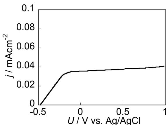
Fig. 20. Photocurrent density versus potential ( $j$ - $U$ ) curve for the multi-photon system (Fig. 17) using the same titanium dioxide thin film and Pt-nanoparticle modified microcrystalline Si photoelectrodes and electrolyte solutions as those in Figs. 18 and 19 under simulated solar light illumination.
