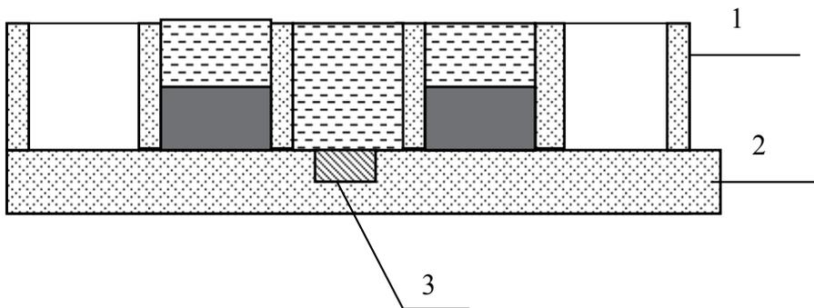
Fig. 4.1. Conventional slide boat for LPE growth: 1, body boat; 2, slider, 3, substrate.
