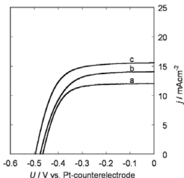
Fig. 10. Photocurrent density versus potential ( $j$ - $U$ ) curves of photovoltaic photoelectrochemical solar cells equipped with Pt-nanoparticle modified multicrystalline n-Si photoelectrode having no porous layer pretreated under the same conditions as the specimens of Fig. 4. Pretreatment: method A (image a), B (b and c); Pt deposition time: 120 (a and b), 30 s (c).
