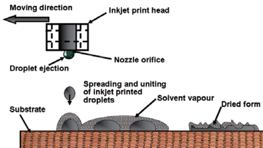
Fig. 5. Inkjet printing of photovoltaic cells
