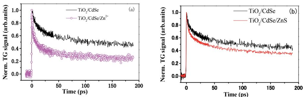
Fig. 9. Transient grating kinetics of CdSe QD adsorbed TiO<sub>2</sub> electrode before and after the surface modification with Zn<sup>2+</sup> (a) and ZnS (b).
