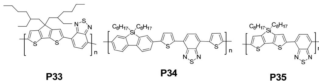
Chart 13. Structures of low band gap polymers P33, P34 and P35
