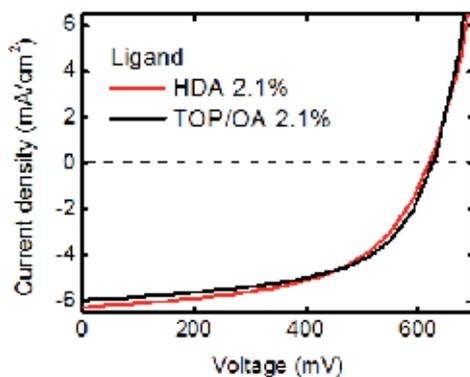
Fig. 6. Comparison of J-V characteristics of the best devices fabricated based on HDA or TOP/OA ligand capped CdSe QDs and P3HT, exhibiting similar PCEs of 2.1%.
