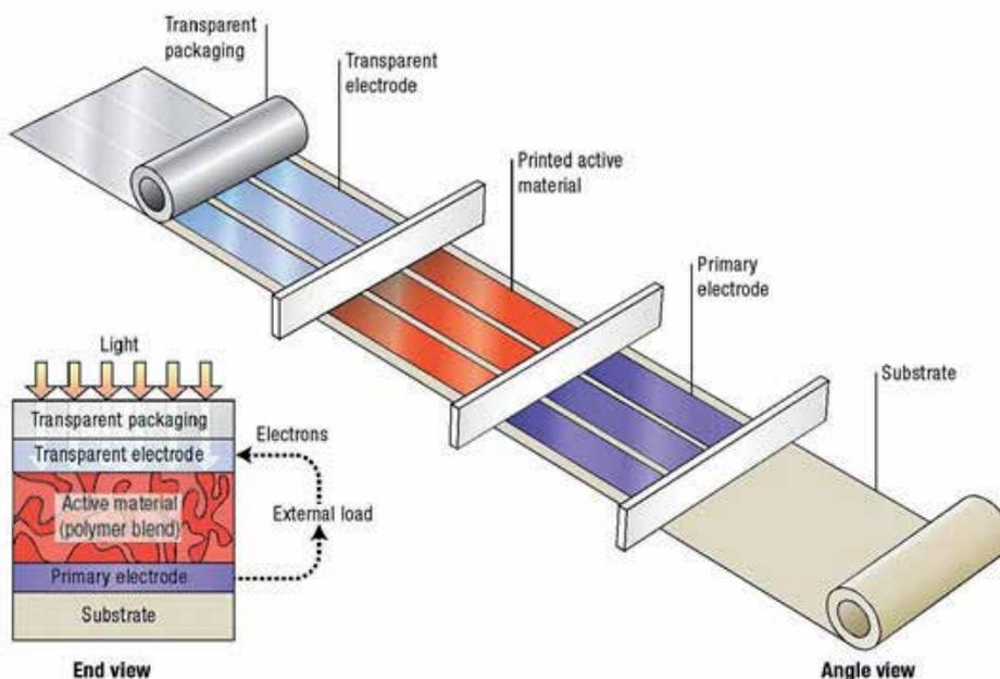
Fig. 3. Schematic description of printing process used for manufacturing of polymer-based photovoltaic cells. Reprinted by permission from Macmillan Publishers Ltd: Nature Photonics, *Gaudiana, R. & Brabec, C.* (2008). Organic materials: Fantastic plastic. Vol.2, pp.287- 289, copyright (2008).
