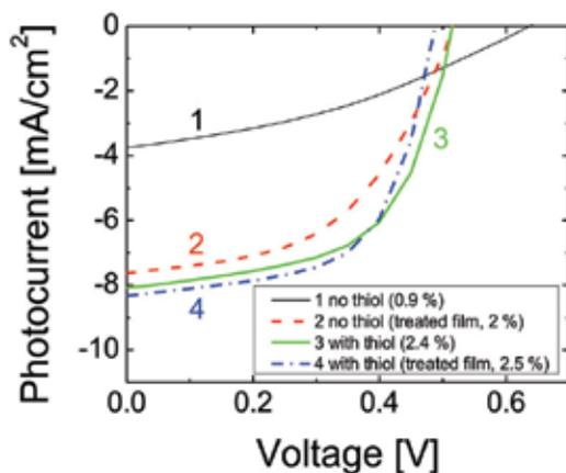
Fig. 15. Current-voltage characteristics demonstrating significant performance improvement under illumination ( $1000 \text{ W/m}^2$ ,  $1.5 \text{ AM}$ ) for P3HT/PCBM bulk-heterojunction solar cells prepared in different ways: as produced (thin line), annealed (thick dashed line), thiol added (thick line), thiol added and annealed (thick dash dot line). Reprinted with permission from (Pivrikas et al., 2008). Copyright 2008, with permission from Elsevier.
