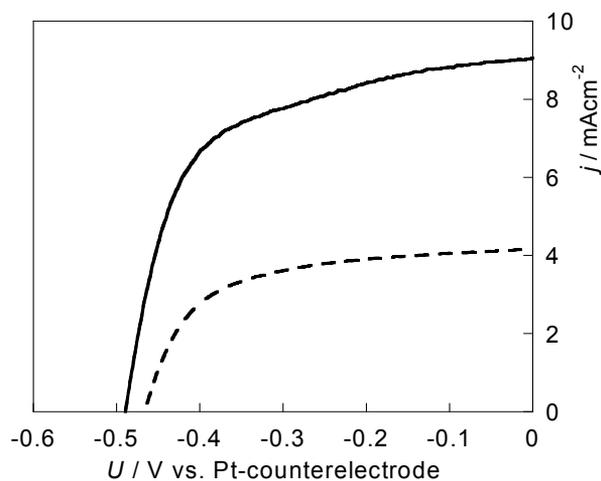
Fig. 15. Photocurrent density versus potential ( $j$ - $U$ ) curves for photovoltaic photoelectrochemical solar cell equipped with the Pt-nanoparticle modified microcrystalline Si photoelectrode measured in the  $7.6 \text{ mol dm}^{-3}$  (M) hydroiodic acid (HI)/ $0.05 \text{ M}$  iodine ( $\text{I}_2$ ) (dashed line) and  $3.0 \text{ M}$  HI/ $0.002 \text{ M}$   $\text{I}_2$  (solid line) redox solutions.
