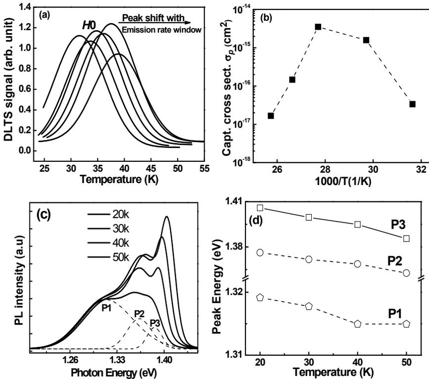
Fig. 10. (a) Emission rate window dependence of  $H0$  peak, (b) temperature dependence of capture cross section and activation energy of  $H0$ , (c) PL spectra of p-type GaAsN at 20 to 50 K, and (d) temperature dependence of the peaks  $P1$ ,  $P2$ , and  $P3$  obtained from the fitting of PL spectra.
