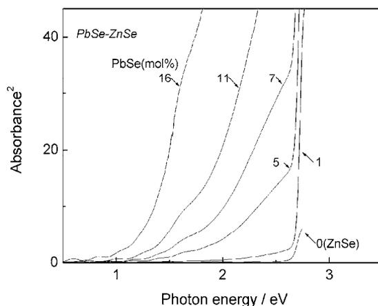
Fig. 3.5. Optical absorption spectra for PbSe/ZnSe composite thin films (after Abe, 2011).
