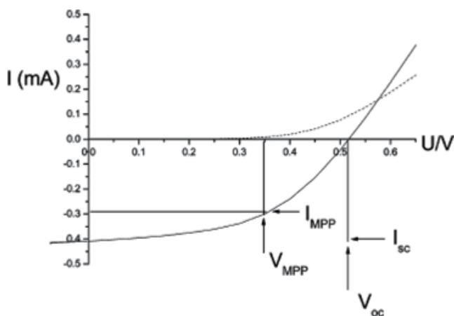
Fig. 4. Current-voltage (I-V) curves of an organic solar cell (dark, - - -; illuminated, -). The characteristic intersections with the abscissa and ordinate are the open circuit voltage ( $V_{oc}$ ) and the short circuit current ( $I_{sc}$ ), respectively. The largest power output ( $P_{max}$ ) is determined by the point where the product of voltage and current is maximized. Division of  $P_{max}$  by the product of  $I_{sc}$  and  $V_{oc}$  yields the fill factor  $FF$  (Günes et al., 2007).
