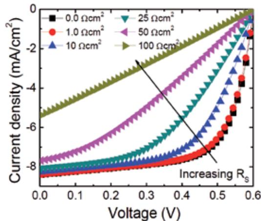
Fig. 12. Effect of  $R_s$  variation on  $J$ - $V$  characteristics of the P3HT:PCBM solar cells according to (1). Only the value of  $R_s$  is changed while keep  $J_0=3.03\text{e-}5 \text{ mA/cm}^2$ ,  $J_{ph}=8.40 \text{ mA/cm}^2$ ,  $R_{sh}=617.28\Omega \text{ cm}^2$  and  $n=1.88$ .  $R_s$  greatly affects  $FF$  and thus the overall  $PCE$ .  $J_0$ ,  $R_{sh}$  and  $n$  only slightly affect  $J_{SC}$  in the value range shown in Table 1.
