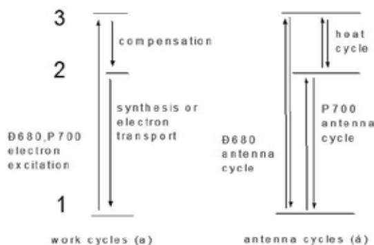
Fig. 13. The interpretation of energy transitions in the work (a) and antenna (b) cycles. Level 1 shows the ground states, levels 2, 3 present excited states of pigment molecules.
