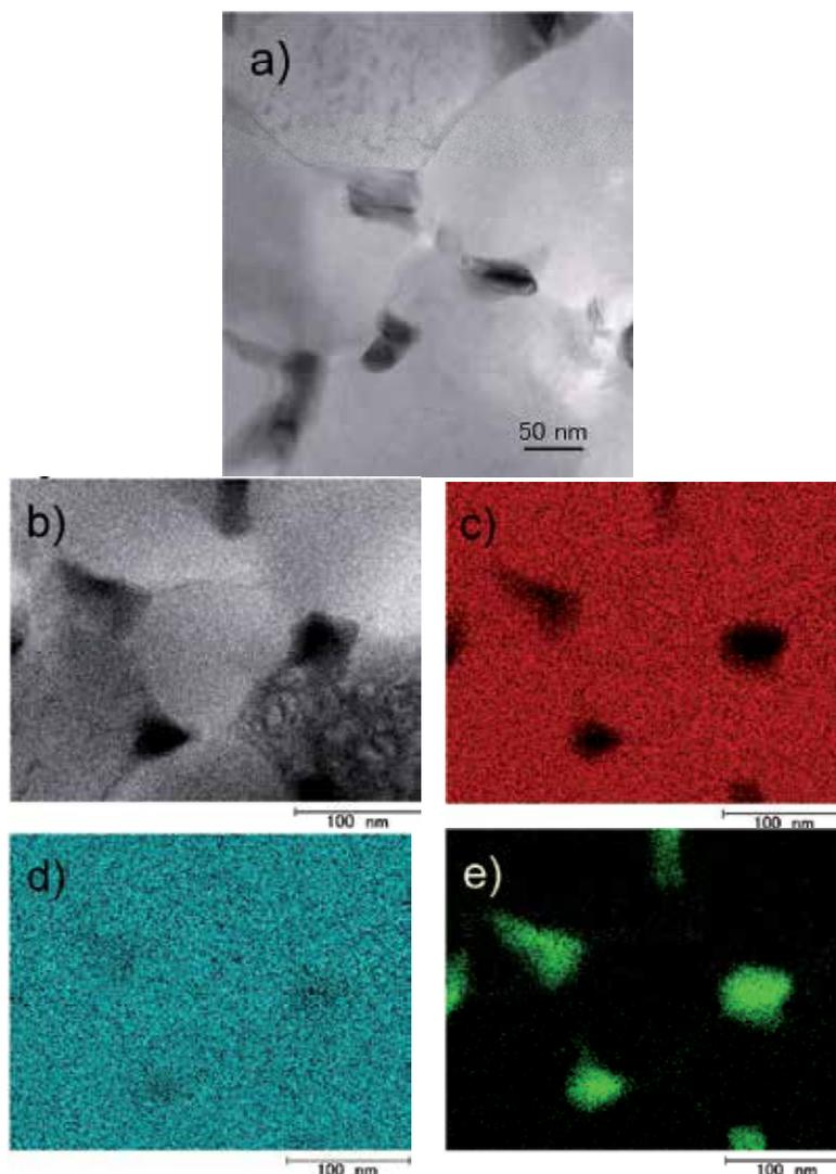
Fig. 3.4. Direct observation of PbSe/ZnSe composite thin film containing 5mol%PbSe. (a) Bright-field TEM image. (b) Bright-field image of STEM mode. (c) Elemental mapping of Zn (red), (d) Se (blue), and (e) Pb (green) (after Abe, 2011).
