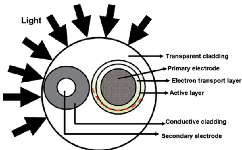
Fig. 3. Photovoltaic fibre
