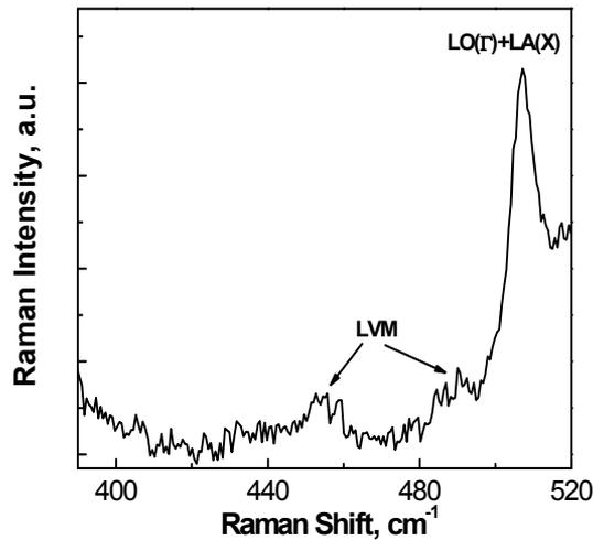
Fig. 5.10. Raman spectrum of as grown InGaAsN layer.
