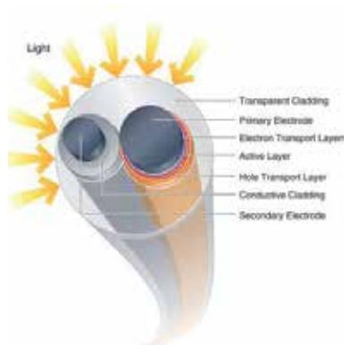
Fig. 15. Schematic of a complete fiber showing the potential for shadowing by the secondary electrode. From Lee, M. R.; Eckert, R. D. ; Forberich, K. ; Dennler, G.; Brabec, C. J. & Gaudiana, R. A. (2009). Solar power wires based on organic photovoltaic materials. *Science*, Vol. 324, pp. 232-235. Reprinted with permission from AAAS.
