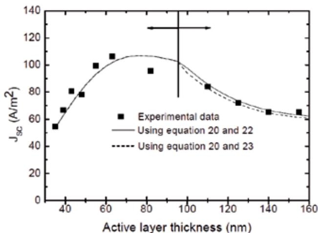
Fig. 7. Short hole carrier lifetime condition. Left arrow: hole lifetime is longer than its transient time; right arrow: hole lifetime is shorter than its transient time, and hole lifetime is  $6.2 \times 10^{-7} s$ , and electron lifetime is  $1 \times 10^{-6} s$ . Experimental data are from [Li et al., 2005].
