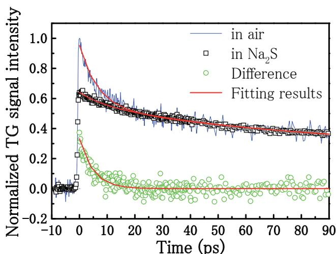
Fig. 3. TG responses of the CdSe QDs adsorbed onto nanostructured  $\text{TiO}_2$  films measured in air (-) and in  $\text{Na}_2\text{S}$  solution ( $\square$ ) as well as their “difference response” ( $\circ$ ) (Shen et al., 2010a).
