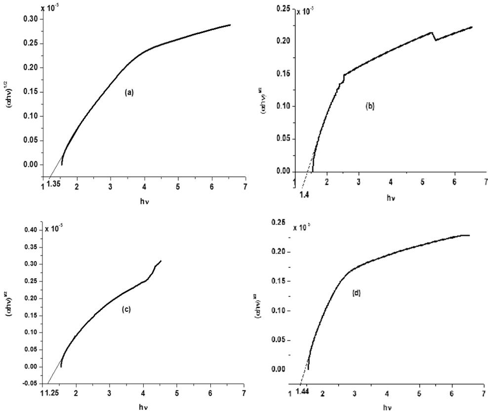
Fig. 5. Bandgap estimation of AlSb semiconductor with Al:Sb growth ratios (a) 1:3, (b) 2:5, (c) 1:1 and (d) 3:7.
