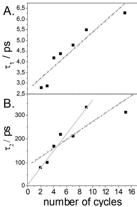
Fig. 6. Dependence of  $\tau_1$  (A) and  $\tau_2$  (B) on the number of SILAR cycles. Dashed lines correspond to linear fittings including all data, whereas the solid line shows a linear fitting forced to pass through the origin without considering the point corresponding to 15 SILAR cycles (Guijarro et al., 2010a).
