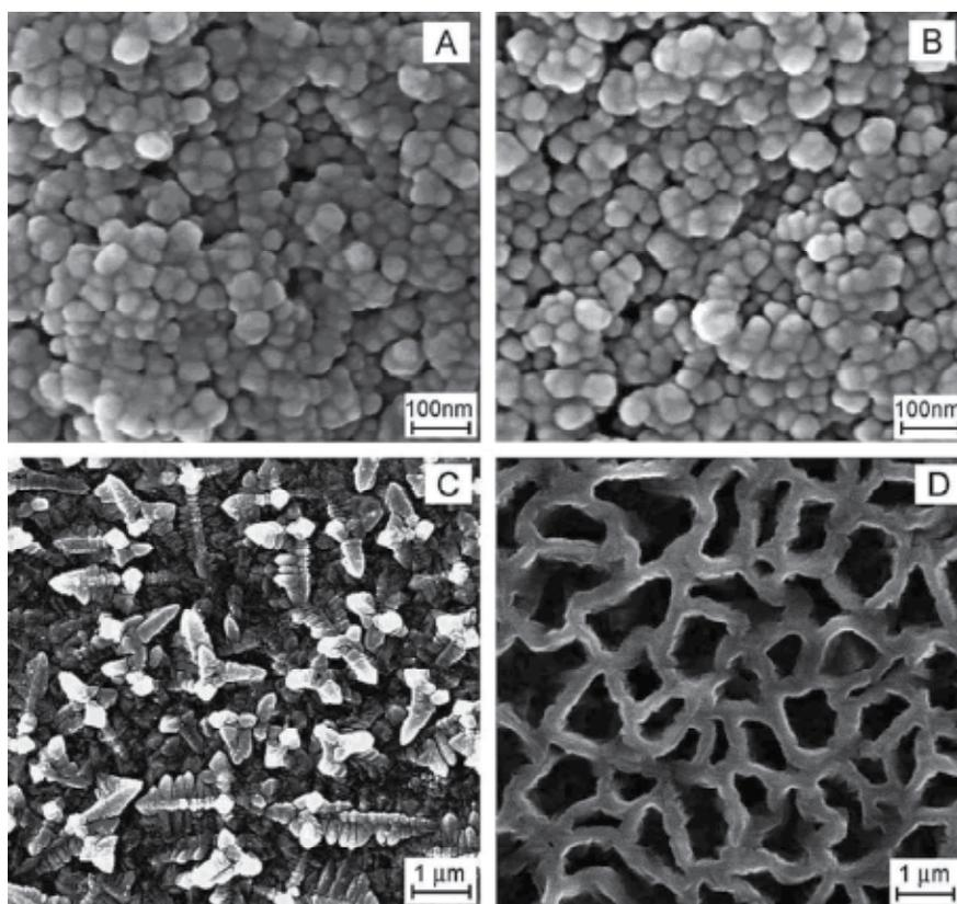
Fig. 4. SEM photographs of  $\text{Cu}_2\text{O}$  films deposited at various bath temperatures: (A)  $0^\circ\text{C}$ , (B)  $30^\circ\text{C}$ , (C)  $45^\circ\text{C}$ , and (D)  $60^\circ\text{C}$  (Tang et al., 2005)
