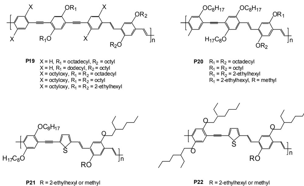
Fig. 16. Chemical structures of acetylene-containing PPV derivatives **P19-P22**
