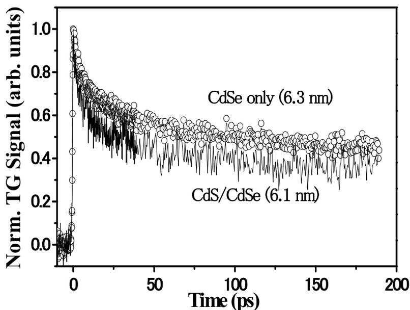
Fig. 10. Ultrafast carrier dynamics of combined CdS/CdSe and CdSe without preadsorbed CdS quantum dots layer with a transient grating (TG) technique.
