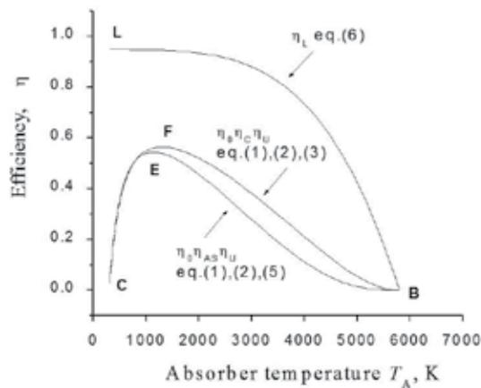
Fig. 9. Comparison of the efficiency  $\mu_L$  of Landsberg engine (the LB line) with the efficiencies of combined engines (the CEB, CFB lines). A difference between the efficiencies  $\eta_0 \eta_{AS} \eta_U$  and  $\mu_O \mu_C \mu_U$  is that in the first case radiation working cycle is not a Carnot cycle. Lines CEB and CFB are practically coincide at temperatures used for operation of solar cells.
