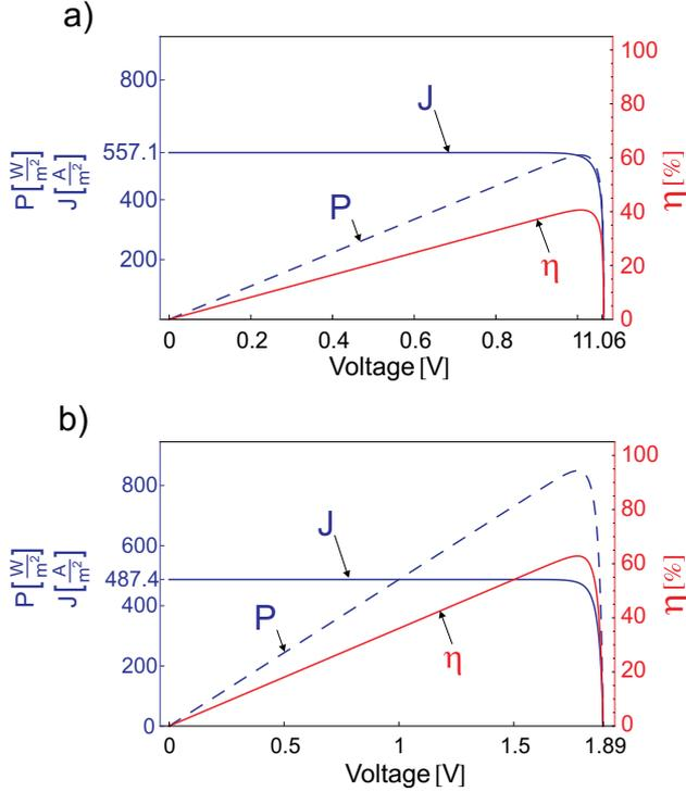
Fig. 5. Voltage dependence of the current density,  $J$ , output power  $P$  and efficiency  $\eta$  for (a) a single-gap solar cell with  $E_G = 1.08$  eV; (b) an intermediate-band solar cell with  $E_G = 1.9$  eV,  $E_{IB} = 0.69$  eV. The cell has a temperature of 300 K; the incident light is characterized by the blackbody radiation at 5760 K and has a maximum concentration. The band alignment corresponds to the maximum efficiency.
