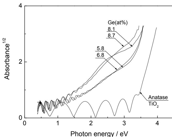
Fig. 2.3. Typical optical absorption spectra of Ge/ $\text{TiO}_2$  composite films with anatase-dominant structure of  $\text{TiO}_2$  matrix (after Abe et al., 2008b).
