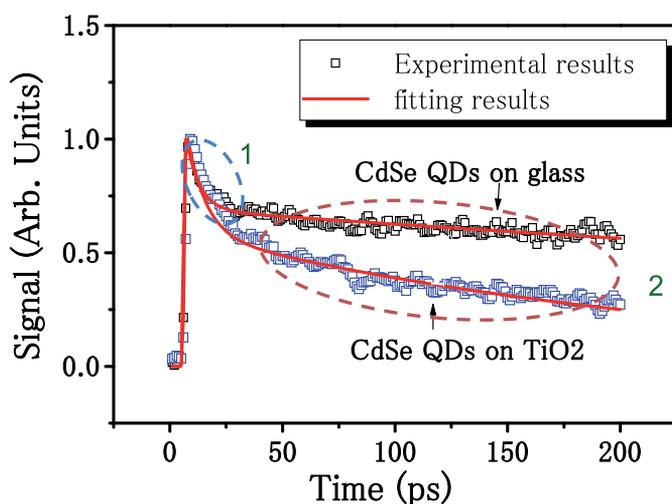
Fig. 4. TG kinetics of the CdSe QDs (average diameter: 5.5 nm) adsorbed on a nanostructured TiO<sub>2</sub> electrode and on a glass substrate under same adsorption conditions (Shen et al., 2008).
