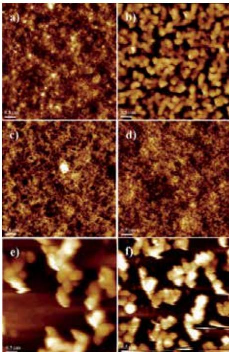
Fig. 11. AFM topography of films cast from PCPCTBT/C71-PCBM with additives: (a) 1,8-octanedithiol, (b) 1,8-dichlorooctane, (c) 1,8-dibromooctane, (d) 1,8-diiodooctane, (e) 1,8-dicyanooctane, and (f) 1,8-octanediacetate. Reprinted with permission from (Chen, Yang, Yang, Sista, Zadoyan, Li & Yang, 2009). Copyright 2009 American Chemical Society.
