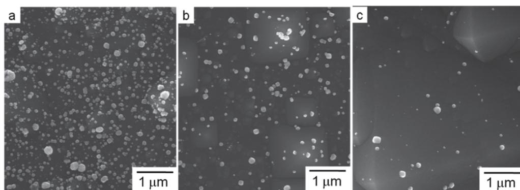
Fig. 4. Typical scanning electron microscopic (SEM) images of multicrystalline n-Si wafers pretreated by method A (image a) or B (b and c) and immersed in the Pt displacement solution for 120 (a and b) or 30 s (c).
