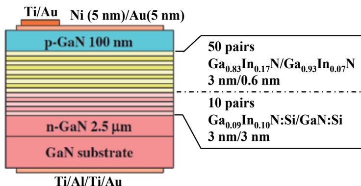
Fig. 1. Schematic of  $\text{In}_x\text{Ga}_{1-x}\text{N}$ -based solar cell exhibiting 2.5% conversion efficiency (Kuwahara, 2011).
