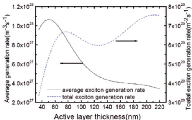
Fig. 3. The calculated exciton generation rate in the active layer when the optical interference effect is considered.
