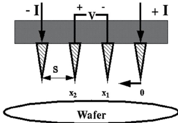
Fig. 6. Schematic diagram of Four point probe configuration.
