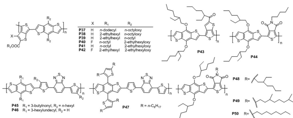
Chart 4. BDT based narrow band gap polymers.
