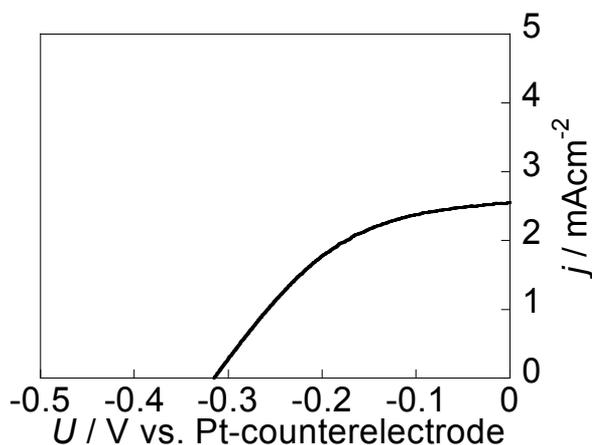
Fig. 19. Photocurrent density versus potential ( $j$ - $U$ ) curve for the photovoltaic photoelectrochemical solar cell equipped with a Pt-nanoparticle-modified microcrystalline Si electrode in the redox solution under simulated solar light illumination through the titanium dioxide photoelectrochemical cell.
