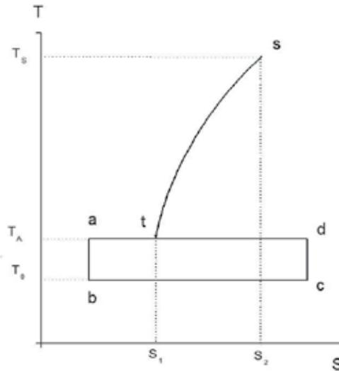
Fig. 2. Entropy diagram showing isochoric cooling of radiation (line *st*) in the cavity 2. The amount of evolved radiant heat is proportional to the area *sts<sub>2</sub>s<sub>2</sub>*. The amount of radiant heat converted into work is proportional to the area *abcd*. The work is performed by matter in a heat engine during Carnot cycle *abcd*.
