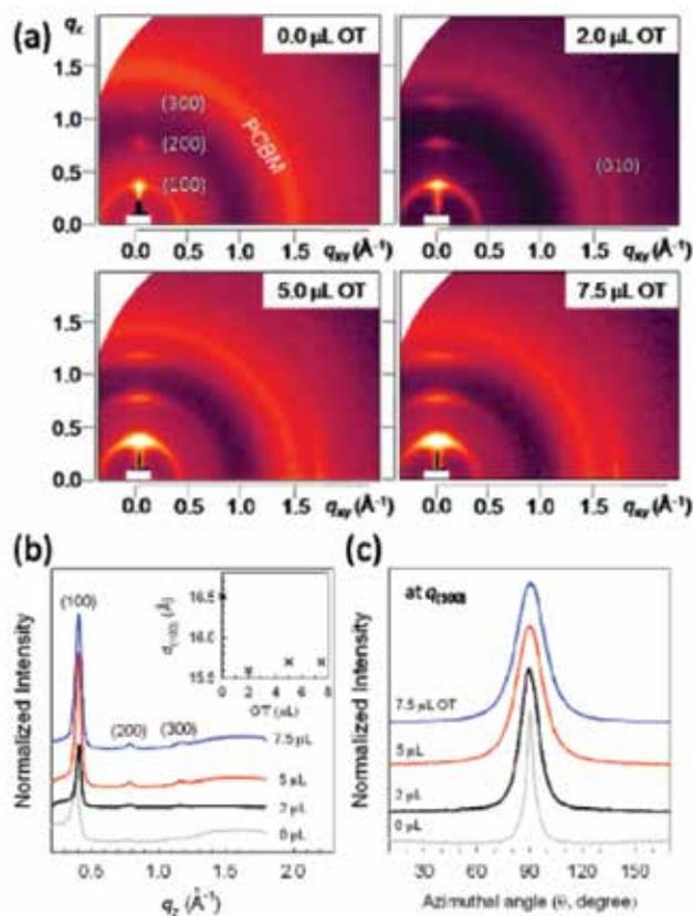
Fig. 13. (a) 2D GIXD patterns of films with different amounts of 1,8-octanedithiol. (b) 1D out-of-plane X-ray and (c) azimuthal scan (at  $q^{(100)}$ ) profiles extracted from (a). Inset of b: calculated interlayer spacing in the (100) direction with various amounts of 1,8-octanedithiol. Reprinted with permission from (Chen, Yang, Yang, Sista, Zadoyan, Li & Yang, 2009). Copyright 2009 American Chemical Society.
