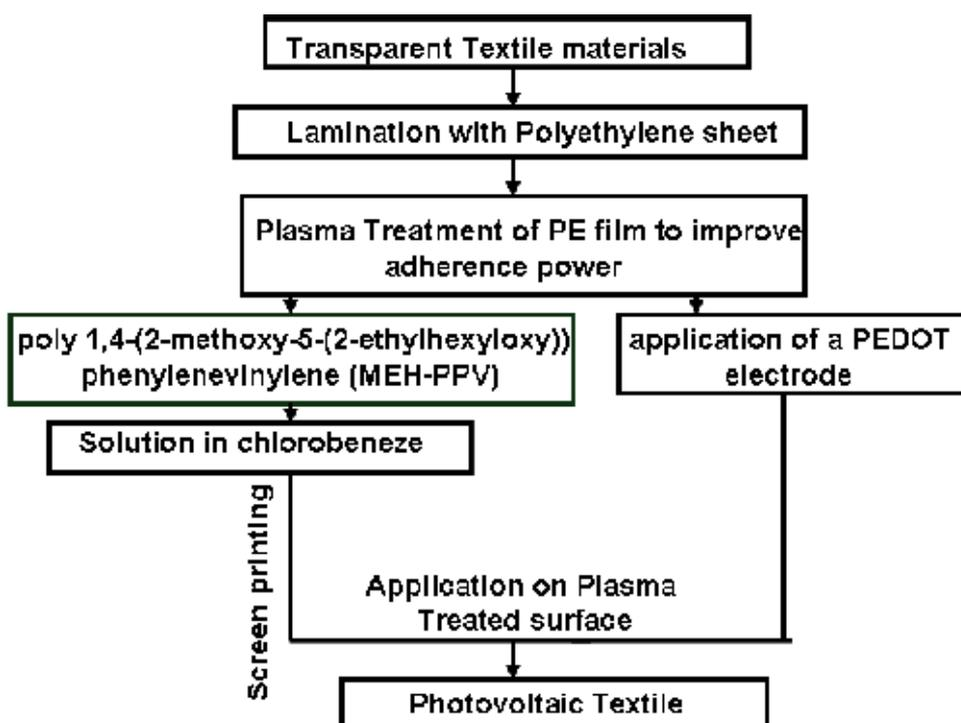
Fig. 2. A typical sequence of photovoltaic textiles manufacturing
