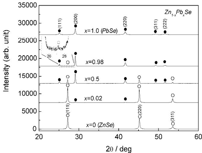
Fig. 3.2. XRD pattern of powder-synthesized  $Zn_{1-x}Pb_xSe$  with respect to  $x$ . Dots indicate PbSe and circles indicate ZnSe (after Abe, 2011).
