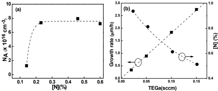
Fig. 13.  $N$  dependence of (a)  $N_A$  and (b) TEGa flow rate dependence of growth rate and  $N$  concentration at a growth temperature of  $420^\circ\text{C}$ .
