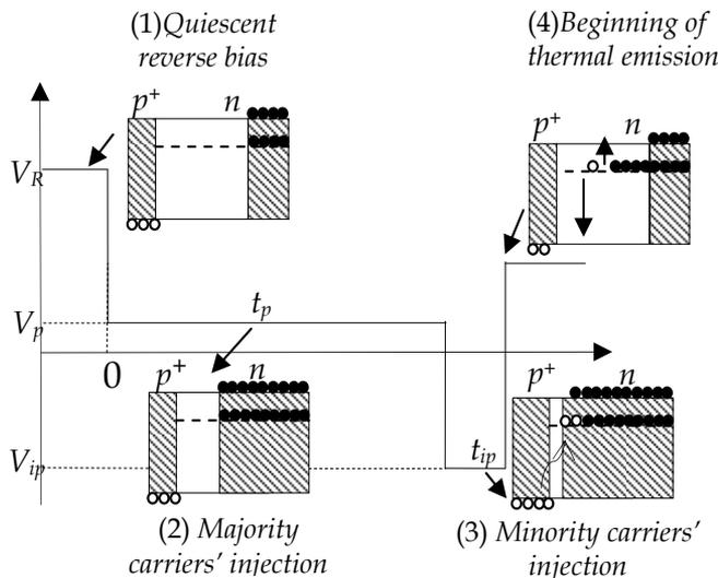
Fig. 1. Basic concept of capture and thermal emission processes from an electron trap located at an energy level  $E_T$  in  $p^+n$  junction. A saturating injection pulse is applied to the reverse biased junction to fill the trap with holes.
