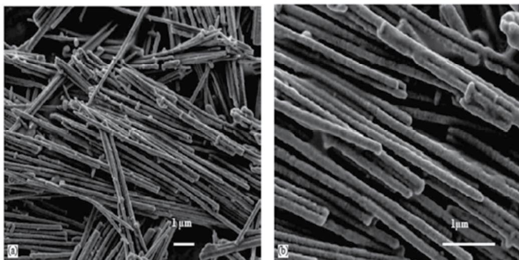
Fig. 3. (a) Scanning electron micrograph of electrodeposited Cu<sub>2</sub>O nanowires. Bath temperature 70°C, pH 9.1, E -1.69 V/SSE. (b) Enlarged (a) (Daltin et al., 2005)
