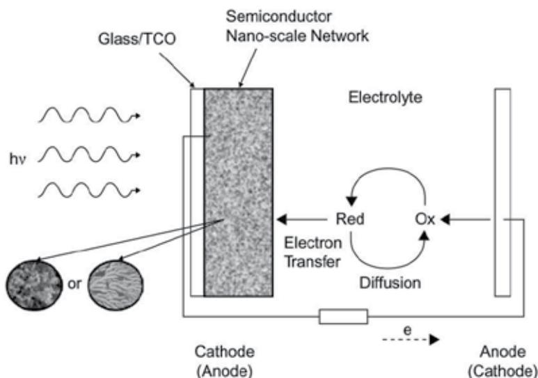
Fig. 2. Schematic of a dye-sensitized SC
