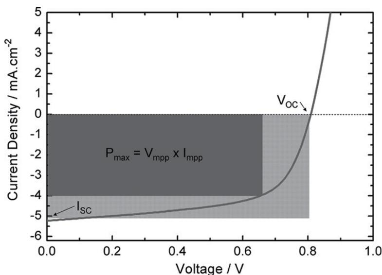
Fig. 4. First and fourth quadrant of a typical  $J$ - $V$  curve observed for a Glass/ITO/PEDOT:PSS/MDMO-PPV:PCBM(1:4)/Al solar cell. Shown are the short circuit current ( $I_{sc}$ ), the open circuit voltage ( $V_{oc}$ ), the current ( $I_{mpp}$ ) and voltage ( $V_{mpp}$ ) at the maximum power point ( $P_{max}$ )
