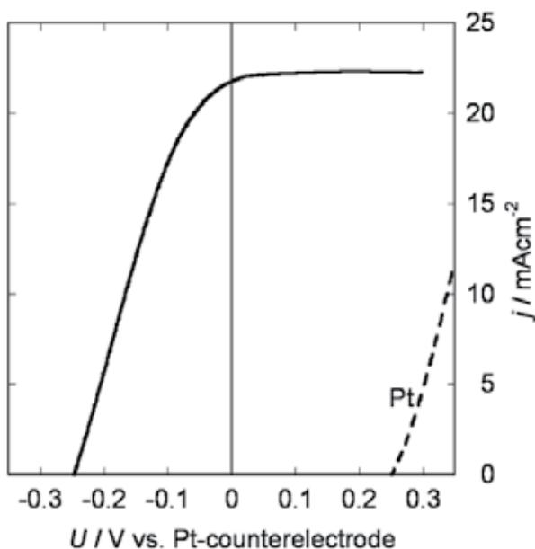
Fig. 12. Photocurrent density versus potential ( $j-U$ ) curve (solid line) for solar-to-chemical conversion type of photoelectrochemical solar cell equipped with Pt-nanoparticle modified porous multicrystalline n-Si electrode prepared under condition g in Table 1. The two-compartment cell for photodecomposition of hydrogen iodide (Fig. 1b) was used. Dashed line: Pt electrode measured in the anode compartment of the two-compartment cell instead of the Si photoelectrode.
