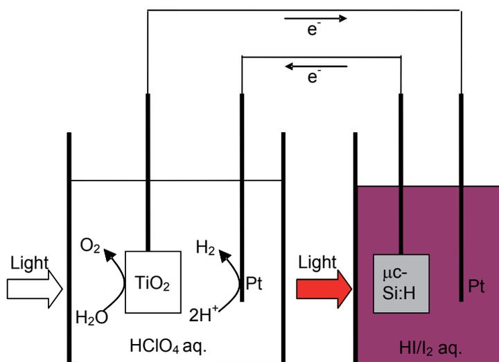
Fig. 17. Schematic illustration of multi-photon system equipped with titanium dioxide and microcrystalline Si photoelectrodes for solar water splitting.
