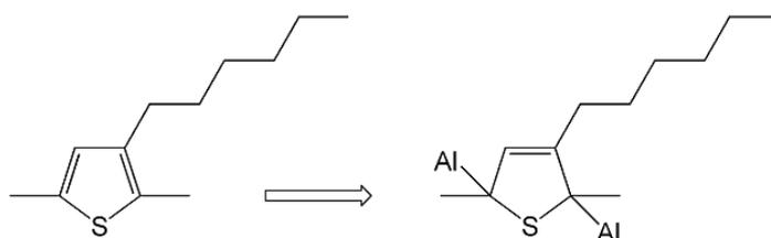
Fig. 11. The proposed molecular structure transits from P3HT to P3HT-Al complex.
