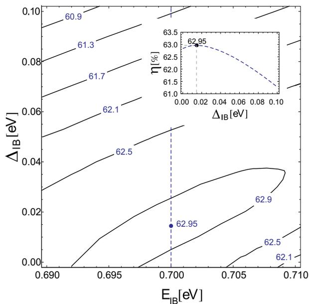
Fig. 7. Detailed balance efficiency of an IBSC with a fixed energy gap  $E_G = 1.90$  eV versus the width  $\Delta_{IB}$  and position  $E_{IB}$  of the intermediate band. In the inset, the profile of the efficiency function across the dashed line in the contour plot is shown.
