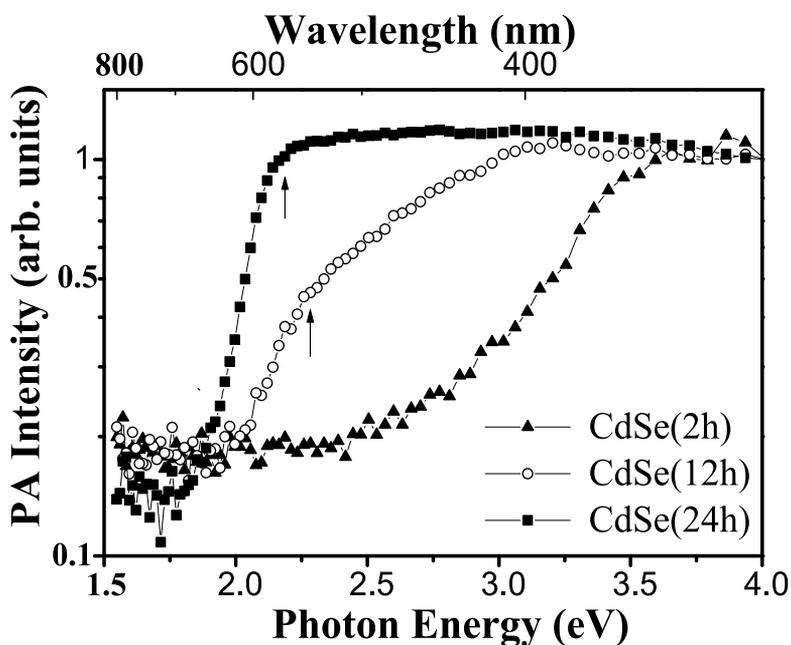
Fig. 3. Photoacoustic spectra of nanostructured TiO<sub>2</sub> electrodes adsorbed with CdSe quantum dots without a preadsorbed CdS quantum dot layer for different adsorption times (modulation frequency: 33 Hz).
