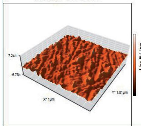
Fig. 5.11. AFM image of the surface of as grown InGaAsN.
