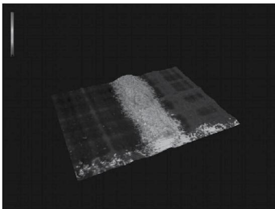
Fig. 15. Contact strip morphology. Scanning area  $430 \times 580 \mu\text{m}^2$ ; magnification 5000x.
