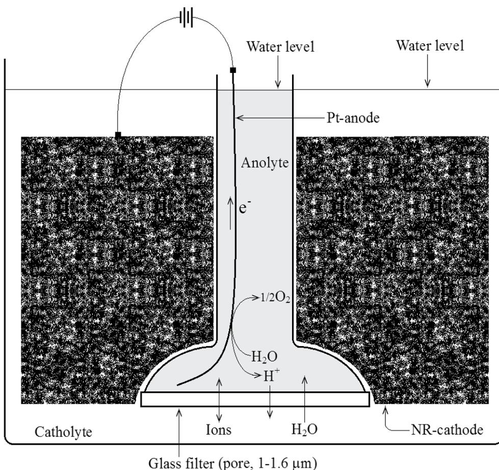
Fig. 5. Schematic structure of the anode and cathode compartment separated by glass filter. Protons, electrons, and oxygen generated from water by the electrolysis may be transferred separately to the catholyte, the NR-cathode, and the atmosphere.
