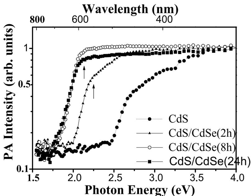
Fig. 2. Photoacoustic spectra of nanostructured TiO<sub>2</sub> electrodes adsorbed with combined CdS/CdSe quantum dots for different adsorption times together with that adsorbed with CdS quantum dots only (modulation frequency: 33 Hz).
