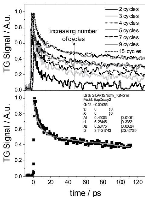
Fig. 5. Transient grating kinetics of CdSe QD adsorbed TiO<sub>2</sub> electrodes with different SILAR cycles (a) and an example of the fitting of the TG kinetics (15 cycles) to a double exponential decay (eq. (3)) (b) (Guijarro et al., 2010a).
