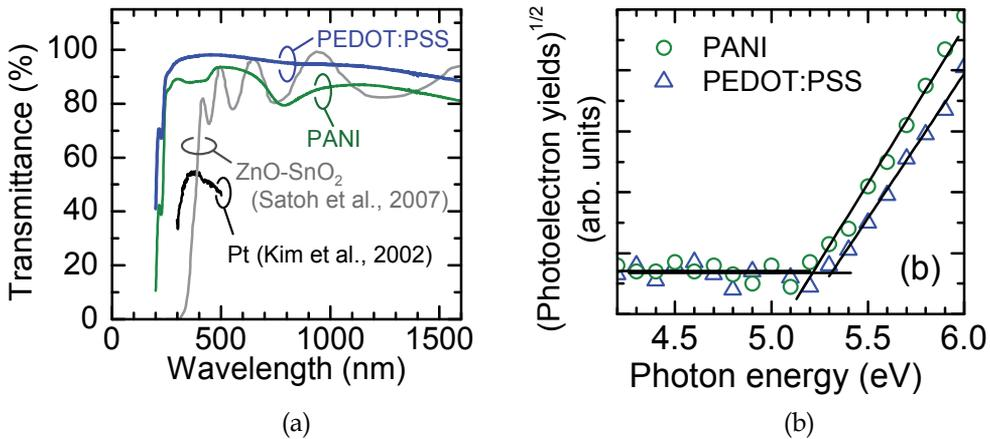
Fig. 3. (a) Optical transmittance spectra of PEDOT:PSS and PANI films. The transmittance spectra of ZnO-SnO<sub>2</sub> (Sato et al., 2007) and semi-transparent Pt (Kim et al., 2002) thin films are also shown for comparison. (b) Photoelectron emission yield spectra of PEDOT:PSS and PANI films.
