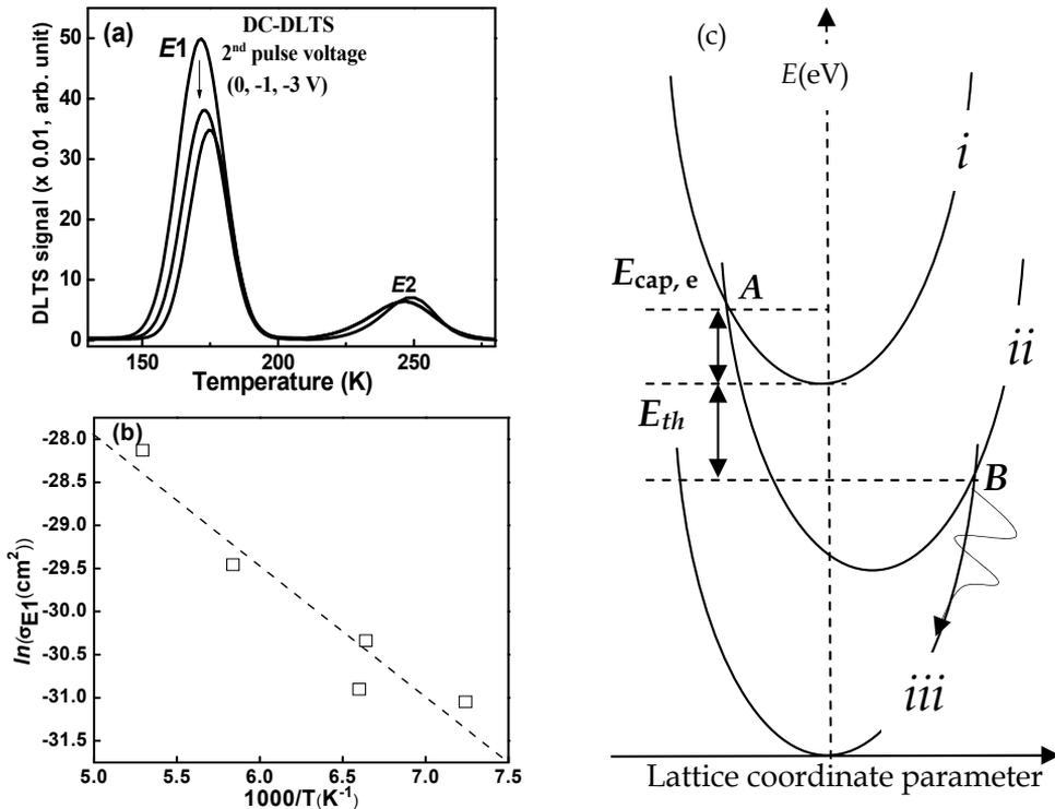
Fig. 5. (a) Reduction of peak height of *E1* under minority carrier injection spectra, (b) temperature dependence of  $\sigma_{E1}$  for electrons, and (c) Configuration-coordinate-diagram showing the different charge states of *E1* as function of lattice coordinate parameter.
