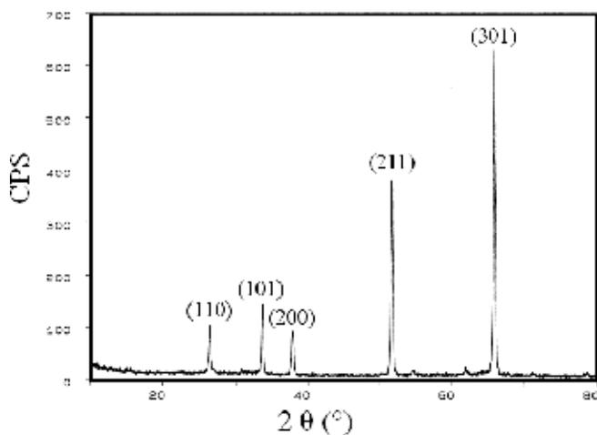
Fig. 9. XRD Diagram of SnO<sub>2</sub> thin layers prepared at T<sub>s</sub> 440 °C.
