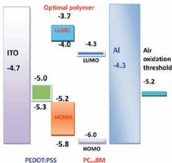
Fig. 2. Optimal HOMO/LUMO energy level of optical polymer used in BHJ solar cell with PC<sub>60</sub>BM as acceptor (Blouin et al., 2008)
