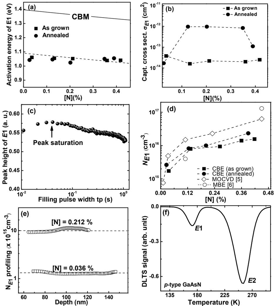
Fig. 3. Nitrogen dependence of (a) thermal activation energy, (b) capture cross section, and (d) adjusted density of  $E1$  in as grown and annealed GaAsN samples. The large capture cross section is confirmed with (c) the filling pulse width dependence of the DLTS peak height of  $E1$ . (e) Density profiling of  $E1$  in the bulk of GaAsN films, and (f) DLTS spectrum of undoped  $p$ -type GaAsN grown by CBE.
