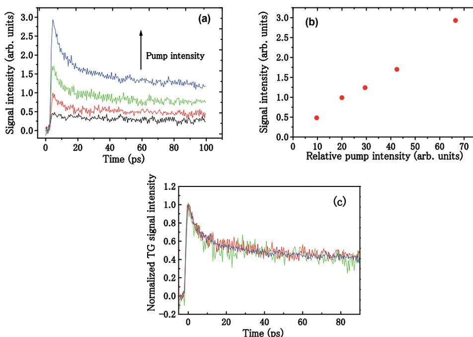
Fig. 1. Dependence of the TG kinetics of CdSe QDs adsorbed onto nanostructured TiO<sub>2</sub> films (CBD method and the CdSe adsorption time was 24 h) on the pump light intensity (a); Dependence of the TG peak intensity on the pump light intensity (b); Normalized TG kinetics measured with different pump light intensities (c) (Shen et al., 2010a).
