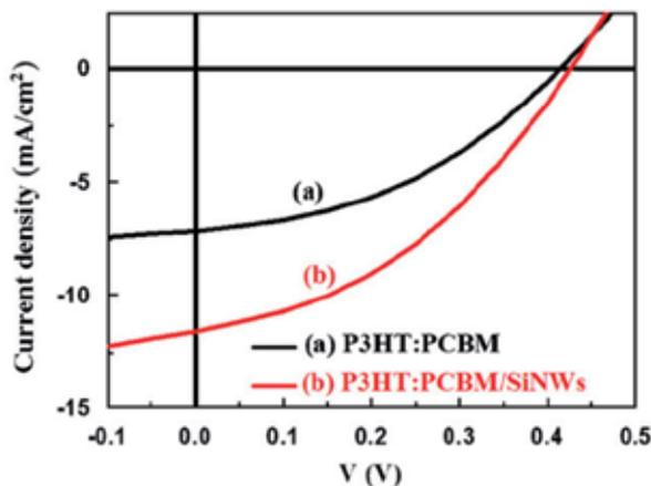
Fig. 5. The current density–voltage characteristics for the SCs with and without the SiNWs under simulated AM1.5 illumination. Reprinted with permission from *Solar Energy Materials & Solar Cells* Vol.93, Huang, J. et al. Well-aligned single-crystalline silicon nanowire hybrid solar cells on glass, pp. 621–624 © 2009, Elsevier.
