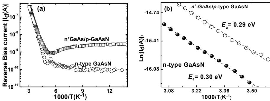
Fig. 4. Temperature dependence of dark current under reverse bias voltages of (a) 0.5 and -0.5V and (b) 1 and -1V in  $n$ -type GaAsN schottky junction and the  $n^+$ -GaAs/ $p$ -GaAsN heterojunction, respectively.
