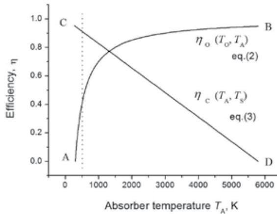
Fig. 3. Efficiencies of Carnot cycles in which the radiation takes place. The efficiency  $\eta_0$  of work of radiation and matter in a cycle with temperatures limited at  $T_0$  and  $T_A$  is shown as curve AB. Line CD shows the efficiency of a cyclic process where work is performed by radiation only.
