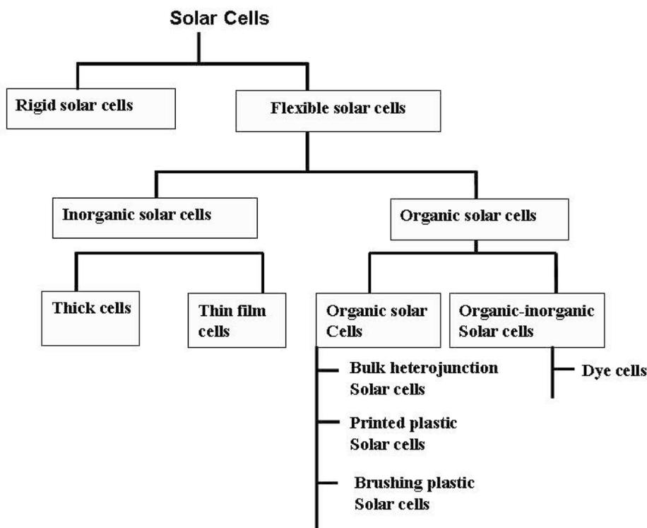
Fig. 1. Classification of Solar cells
