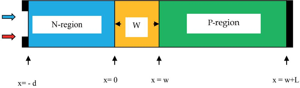
Fig. 3. Typical modeling geometry of a solar cell:  $w$  is the depletion width,  $J$  is the exact interface,  $L$  is the width of the p-region and  $d$  is the n-region (window layer). Note that the n-region is the window for solar photons.
