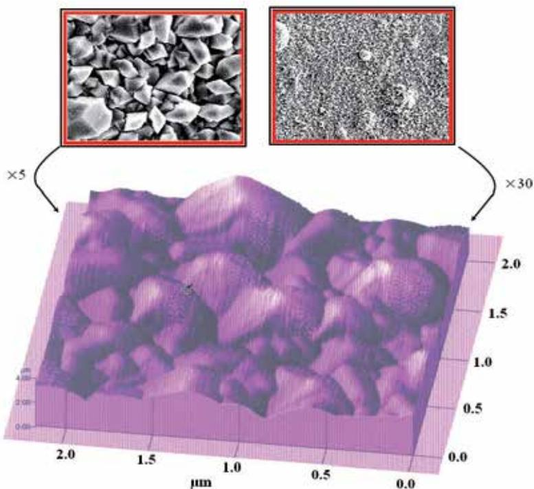
Fig. 10. SnO<sub>2</sub> layers 3D and 2D surface topography 2D (top) and 3D (bottom).
