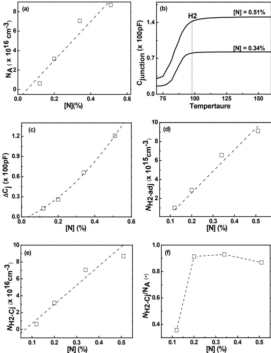
Fig. 12.  $N$  dependence of (a)  $N_A$ , (c) amplitude of  $C_j$  after thermal ionization of  $H2$ , and (d)  $N_{H2\text{-adj}}$ . (b) Sigmoid increase of  $C_j$  between 70 and 100 K for two different GaAsN samples.  $N$  dependence of (e)  $N_{H2-Cj}$  and (f)  $N_{H2-Cj}/N_A$ .
