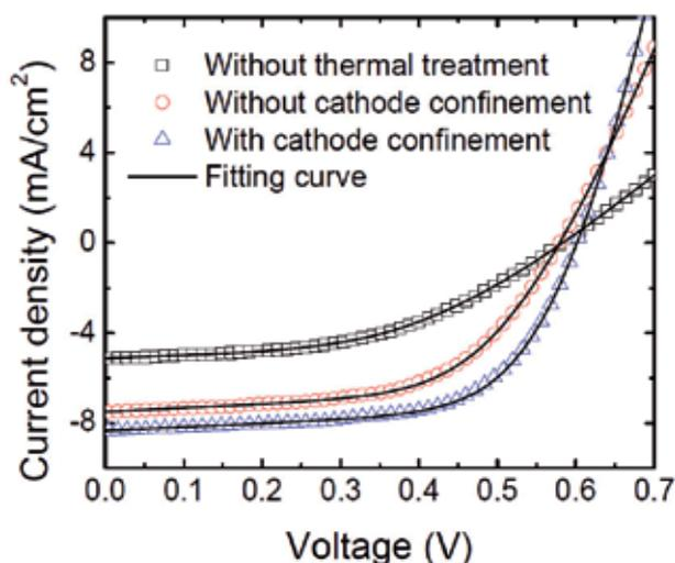
Fig. 9.  $J$ - $V$  characteristics of the solar cells under the AM 1.5 illumination with the light intensity of  $100 \text{ mW}/\text{cm}^2$ . The devices without (circle) and with (triangle) the cathode confinement in the thermal treatment and the device without any thermal treatment (squire) are shown in the graph. Solid lines are the fitting curves according to equation (24).
