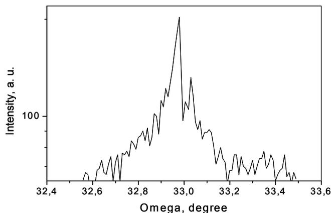
Fig. 5.9. XRD rocking curves of InGaAsN sample
