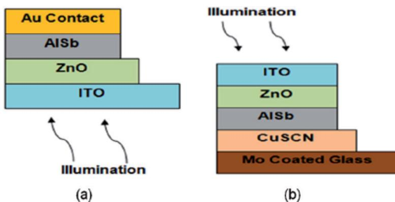
Fig. 9. Solar Cell Design (a) p-n and (b) p-i-n structure.
