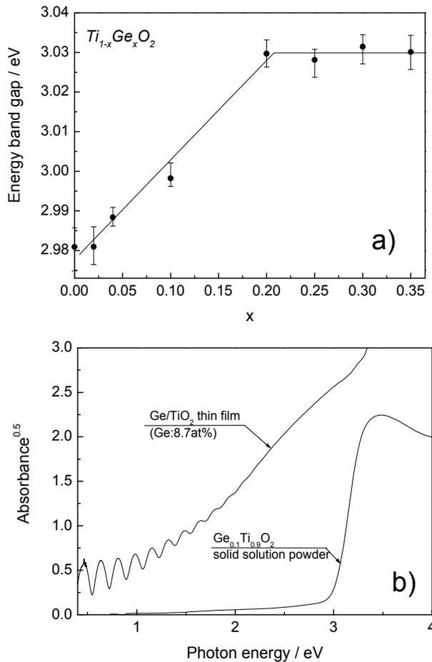
Fig. 2.7. (a) Energy band gap of  $\text{Ti}_{1-x}\text{Ge}_x\text{O}_2$  solid solution at room temperature vs Ge concentration. (b) Absorption spectra of the  $\text{Ge}/\text{TiO}_2$  thin film and a solid solution of the  $\text{Ti}_{1-x}\text{Ge}_x\text{O}_2$  powder (after Abe, 2009).
