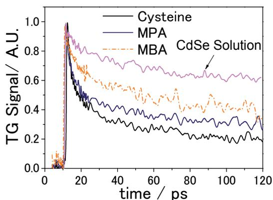
Fig. 7. TG kinetics for CdSe-sensitized TiO<sub>2</sub> electrodes using cysteine, MPA and MBA as linkers. All the curves are normalized to the maximum value. The TG kinetics corresponding to the CdSe solution used for LA adsorption is also given for comparison (Guijarro et al., 2010b).
