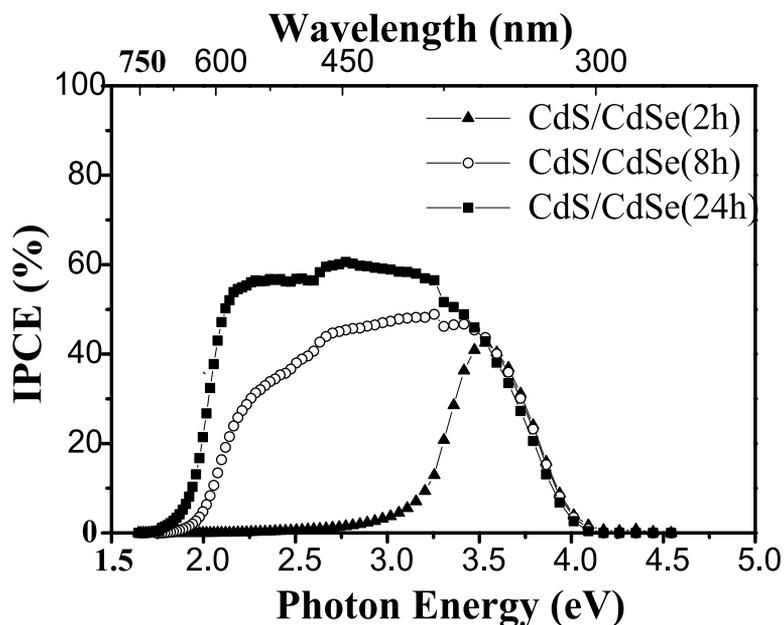
Fig. 6. IPCE spectra of nanostructured TiO<sub>2</sub> electrodes adsorbed with CdSe quantum dots without a preadsorbed CdS QD layer for different adsorption times.
