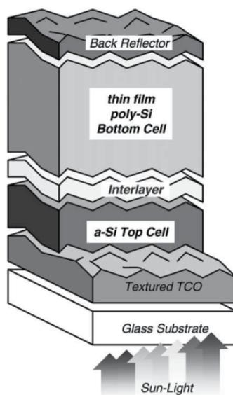
Fig. 8. Schematic view of a-Si/poly-Si ( $\mu$ c-Si) stacked cells with an interlayer. Reprinted with permission from Solar Energy Vol. 77, Kenji Yamamoto et al., A high efficiency thin film silicon solar cell and module, pp. 939–949 © 2004, Elsevier.
