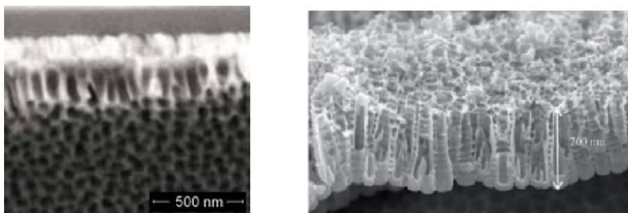
Fig. 11. Left: Side view SEM image of a porous AAO membrane manufactured by anodic oxidation of aluminium at 40 V in the presence of 0.3 M oxalic acid; right: Side view SEM image of porous TiO<sub>2</sub> nanotubes fabricated by anodization of titanium. (Macák et al., 2005). Copyright Wiley-VCH Verlag GmbH & Co. KGaA. Reproduced with permission.
