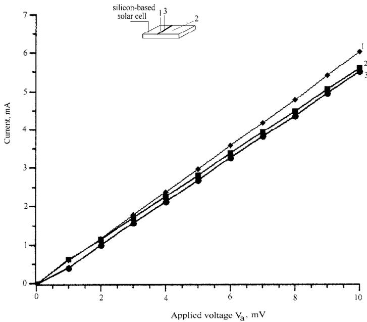
Fig. 18. Room-temperature current-voltage characteristics of the investigated structures <8see text above): functions 1 and 2 are “forward” and “reverse” currents of the MIS-structure (contacts 1-2), and the function 3 is a IVC for the contacts 1-3.
