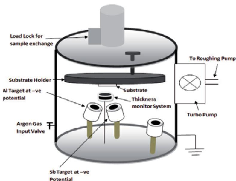
Fig. 2. Schematic diagram of dc magnetron sputtering of Al and Sb targets.
