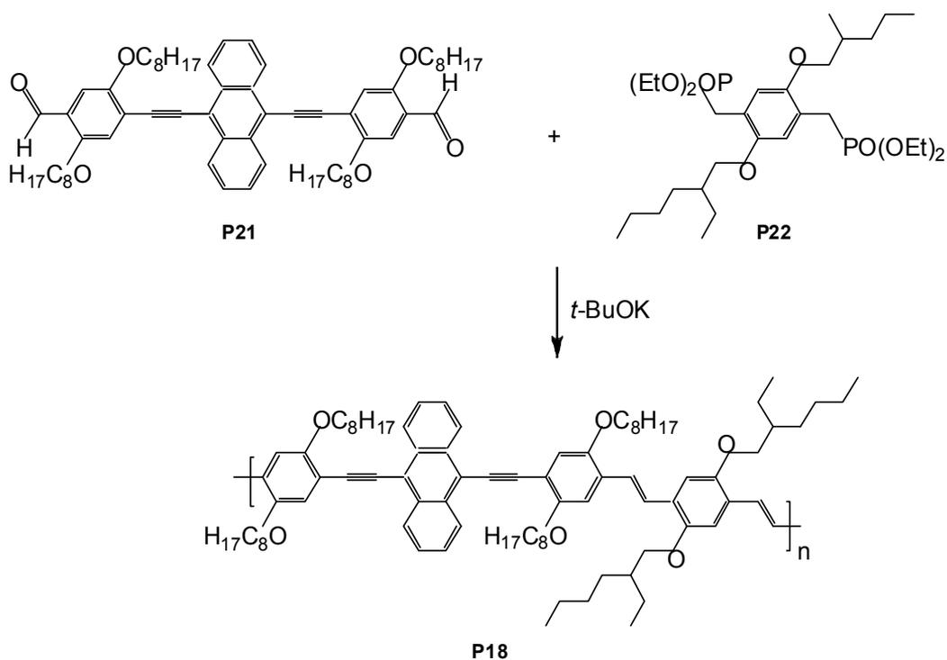
Fig. 15. Synthesis of acetylene-containing **P18** via a Wittig – Horner reaction
