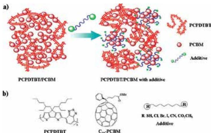
Fig. 9. Schematic depiction of the role of the processing additive in the self-assembly of bulk heterojunction blend materials (a) and structures of PCPDTBT, C<sub>71</sub>-PCBM, and additives (b). Reprinted with permission from (Lee et al., 2008). Copyright 2008 American Chemical Society.
