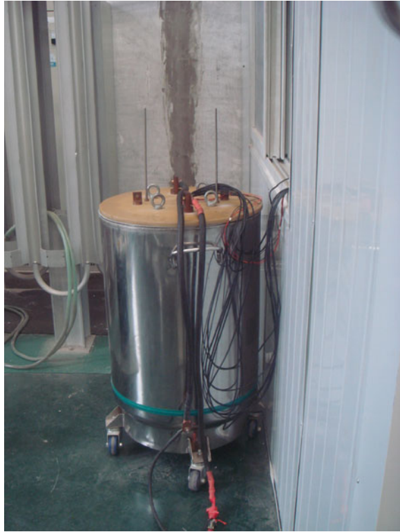
Fig. 6.12 Dewar containing coil with instrumentation connections
