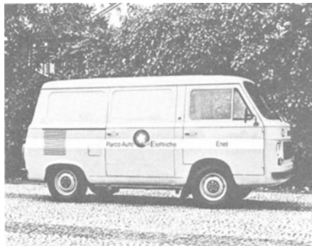
Fig. 11. FIAT-ENEL 900 T Electric Van belonging to an experimental fleet used for activities connected with construction and maintenance of urban distribution networks: maximum speed is 55 km/hr, urban range of 50 km.
