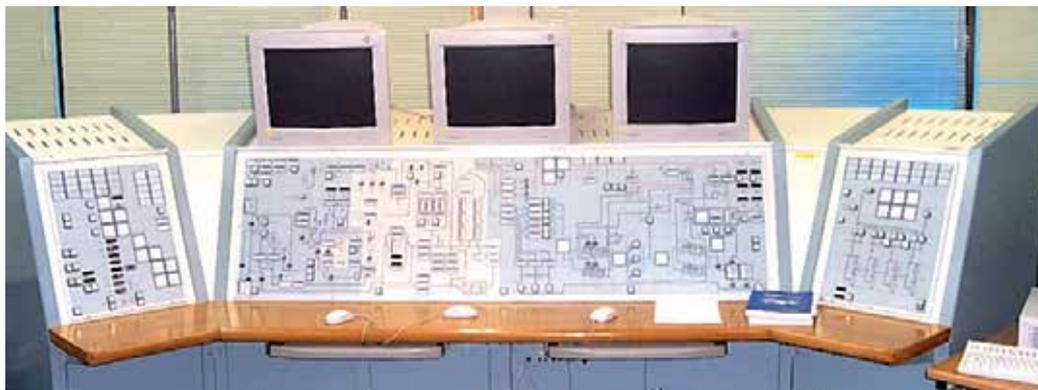
Fig. 2. Reduced-scale full-scope NPP simulator<sup>2</sup>.
