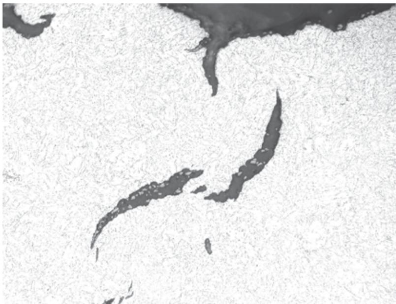
Fig. 8. The occurrence of transverse microcracks on fracture surface and in process zone of the growing crack (Matocha,K., Rožnovská,G. & Hanus,V, 2007).
