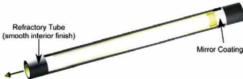
Fig. 9. Hollow-Core Light Guide Concept.
