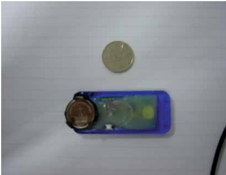
Fig. 2. The size comparison of wireless accelerometer sensor module
