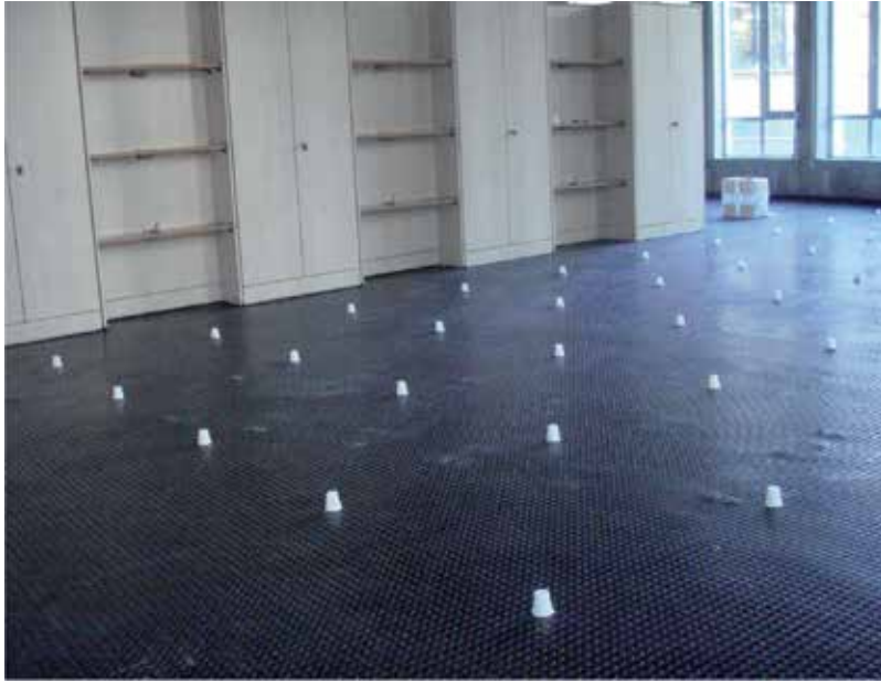
Fig. 7. Deployed testbed using CrossBow's MICAz sensor nodes for ranging calibration.
