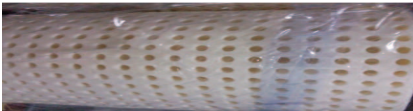
Figure 3. Latex component (Latex): length 1.9 m and 5.1 m; density 147.37\text{ (kg/m}^3\text{)} ; weight 7 kg, thickness 0.02 m.
