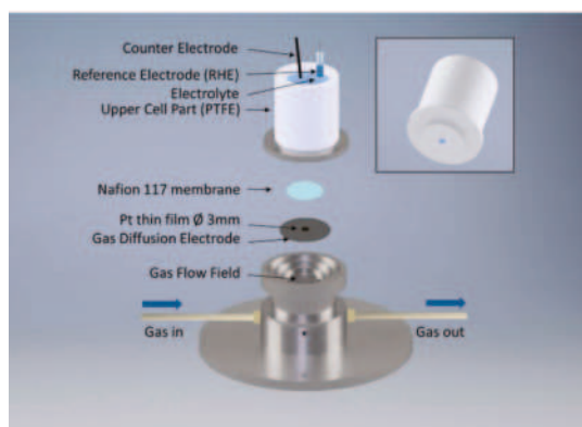
Figure 1. Schematic illustration of the gas diffusion electrode (GDE) half-cell setup, showing the catalyst layer and membrane sandwiched between the upper PTFE with electrolyte and the lower stainless steel body with the gas flow field.
