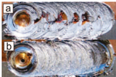
Figure 23. Comparison between a weld with defects (a) and one without defects (b).
