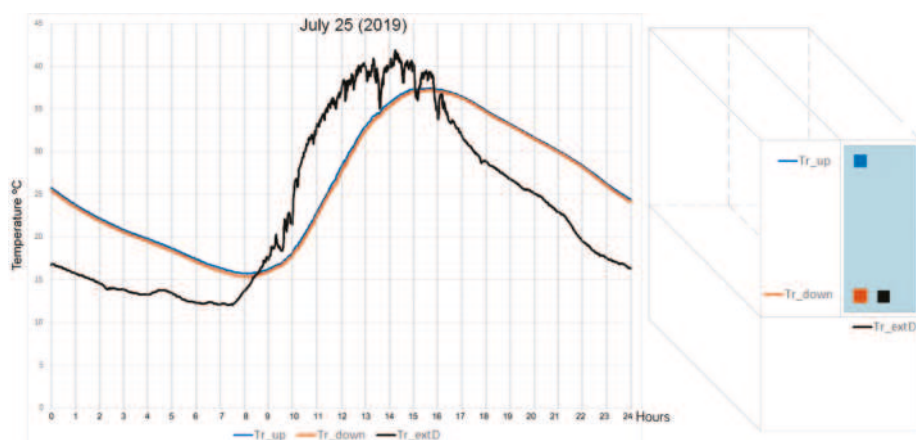
Figure 10. Temperatures of the Reference glazing, both on the outside ( T_{r\_extD} ) and the inside face of the glazing ( T_{r\_up} , T_{r\_down} ). Sample day 25 July 2019.
