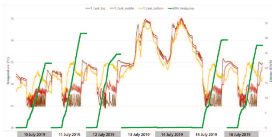
Figure 11. Tank temperatures and heat pump thermal power—sample summer week from 1 July 2019 to 16 July 2019.
