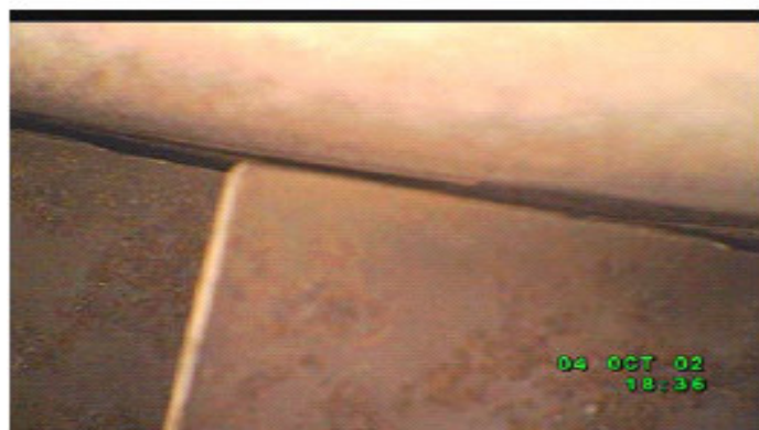
Trailing edge tip rubs & rounding on 13 stage Stator vanes.
