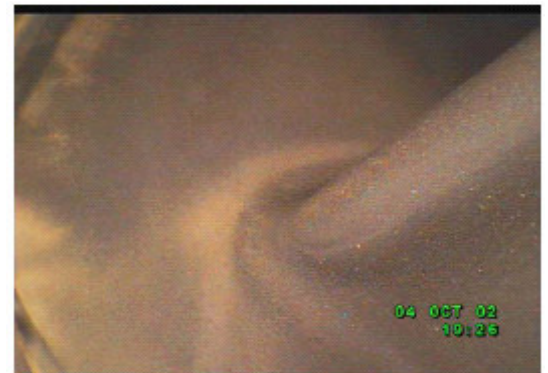
I Stage Nozzle Leading edge & sidewall
