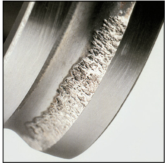
FIGURE 14: SPALLING ON A BEARING RACEWAY
