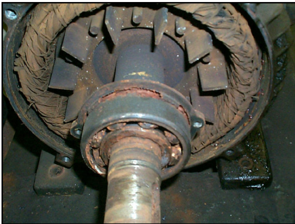
Severe rust has formed on the inside surfaces of this motor.
