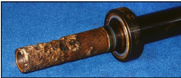
This pump shaft has been damaged by severe cavitation.
