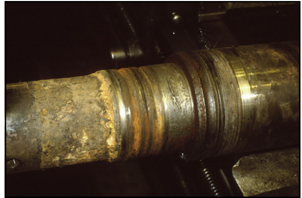
This is an example of severe corrosion on the shaft, due to seal failure. This allowed water to enter into the motor.
