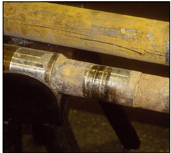
This is a pump shaft with considerable rust damage.
