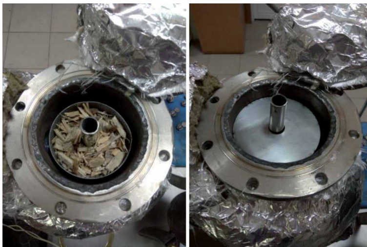
Figure 12. Loading the basket into the pyrolysis chamber and activation.
