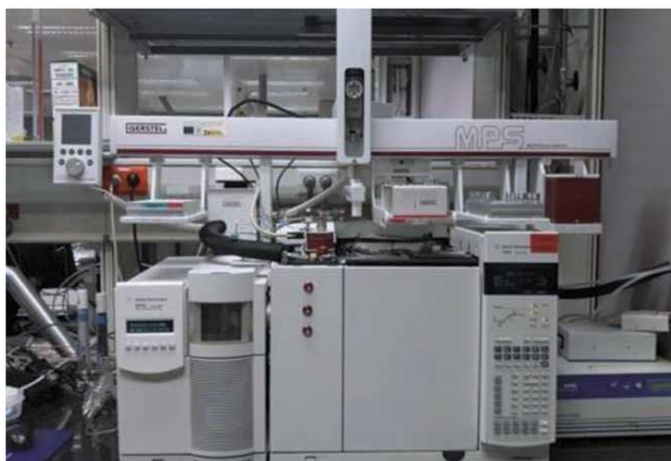
Figure 1. GC/MS with a MultiPurpose sampler (MPS), thermal desorption unit (TDU) and pyrolysis module (PYRO).
