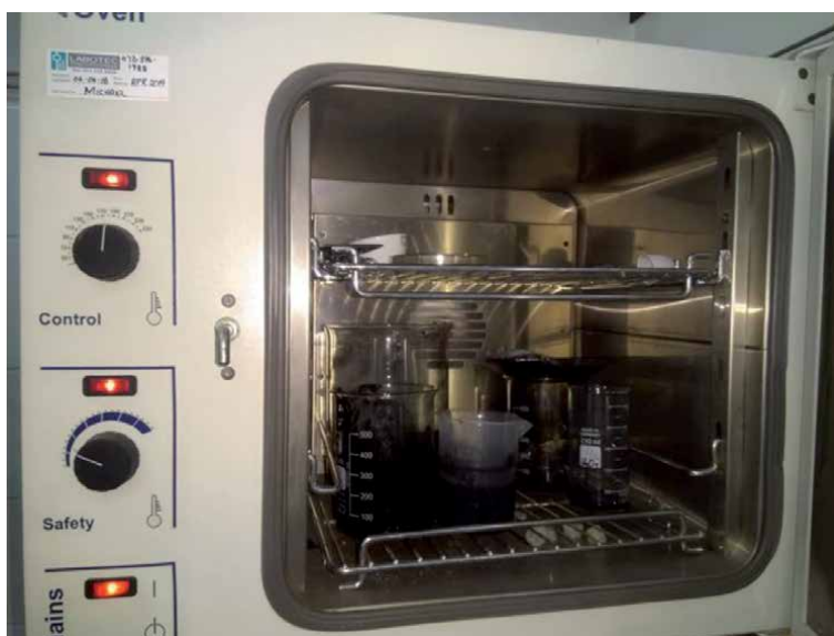
Figure 2. Samples of raw carbon black in an electric oven for chemical activation.
