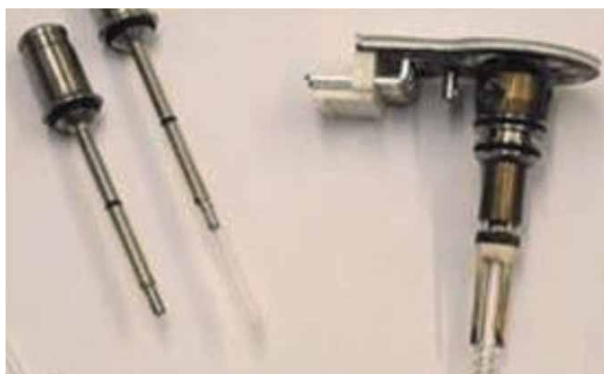
Figure 2. Pyrolysis module with platinum filament, transport adapters and sample holders (Gerstel).
