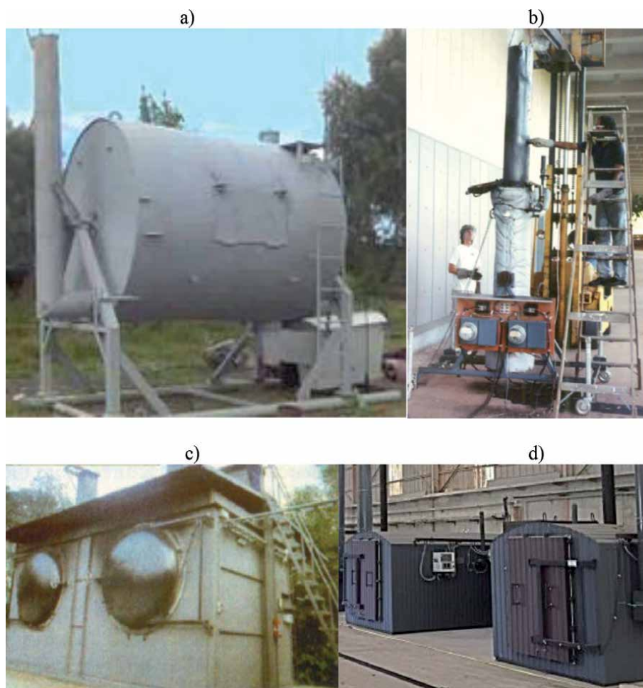
Figure 2. Equipment for the production of charcoal: (a) combustion furnace VMR (USA); (b) experimental reactor Antala (University of Hawaii, USA); (c) UVP-5US mobile incinerator (CIS); (d) charcoal kiln unitary enterprise "EKO-CARBON" (Ukraine).
