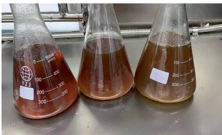
Figure 5. The pyrolysis oil of PP plastic granules.
