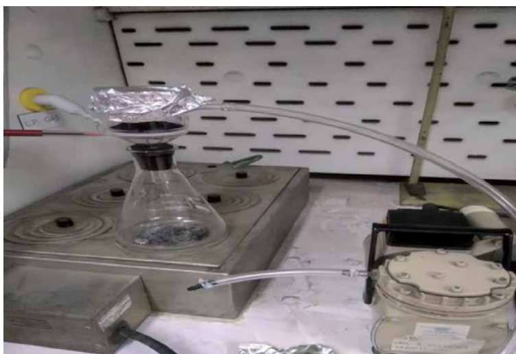
Figure 3. Experimental set up for the extraction generation and adsorption of mercury vapor on the developed AC from waste Tyre pyrolysis. (a peristaltic vacuum pump connected to the filter unit to extract the mercury vapor under the fume wood cupboard).
