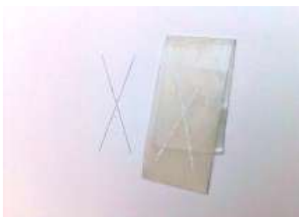
Method A - X-Cut Test and Adhesion Tape
