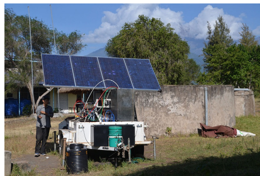
Figure 6. Testing of the PV-powered NF/RO system at the NDRS.
