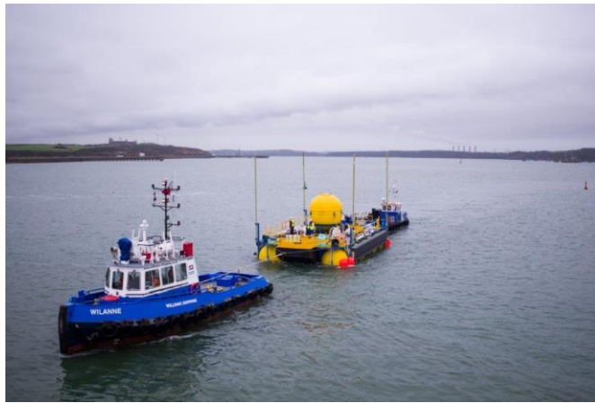
Figure 1: Single float WaveSub on tow, showing the reaction barge in surface configuration with float parked in centre. (Single column image)
