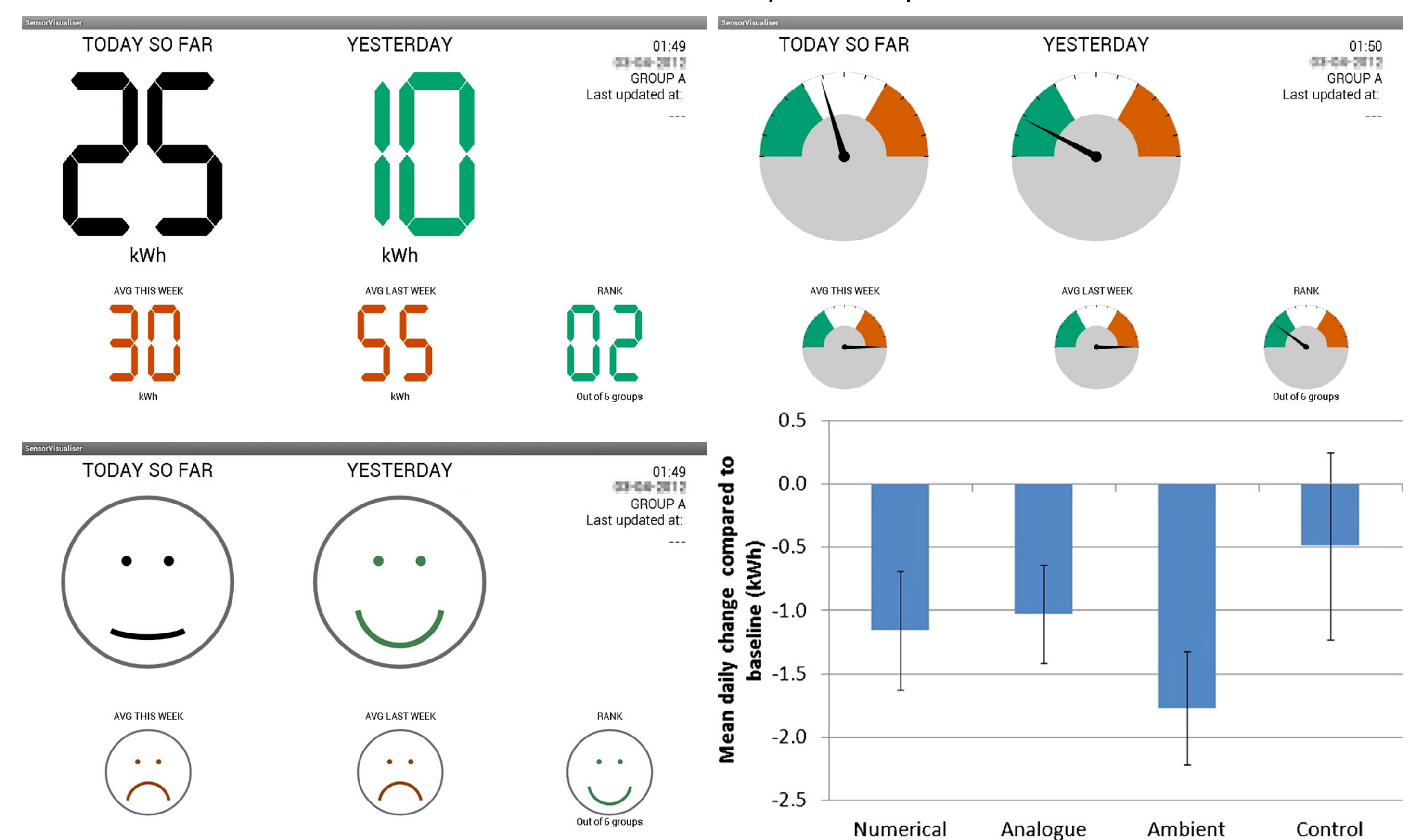
Figure 4: Numerical, analogue and ambient IHD designs and their relative effectiveness. All work well in influencing behaviour [4].
