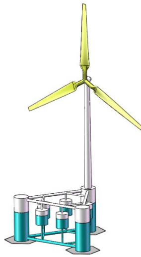
Fig. 2 Hybrid system of a floating wind platform and multiple heaving WECs
