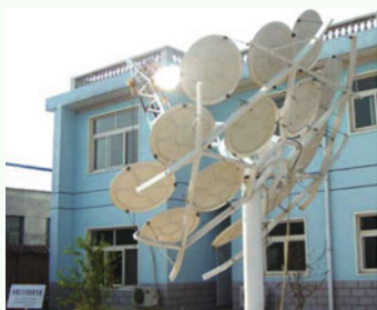
Fig. 2 Multi-dish concentrator developed by Institute of Electrical Engineering, Chinese Academy of Sciences
