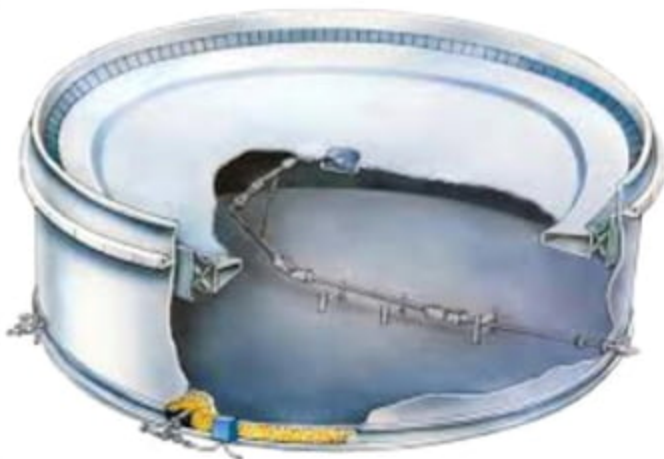
External Floating roof
