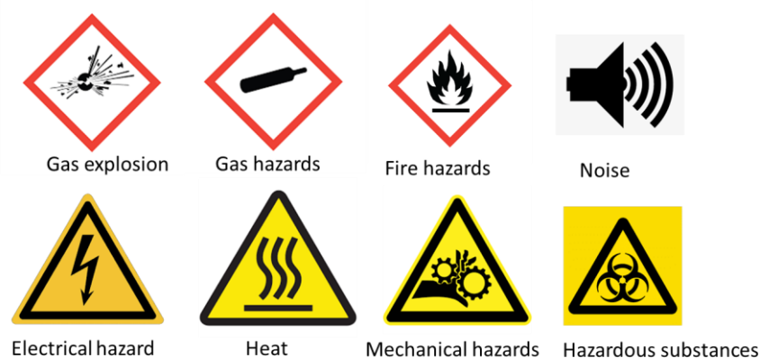
Figure 15 Hazards of the biogas plant.
