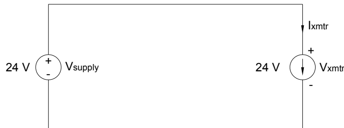
Voltage Drop in an Analog Input Loop Figure A-2
