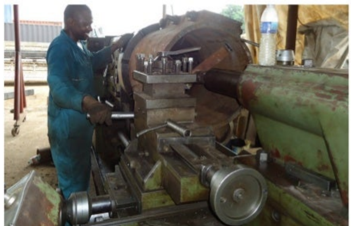
► Valve machining process using a Lathe Machine
