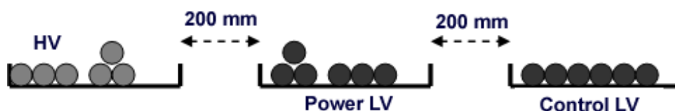
Figure 86: Horizontal distances between cable trays
