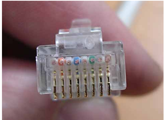
Figure 75: Cable fully home in the connector
