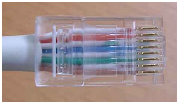
Figure 73: Slide the cable into the connector
