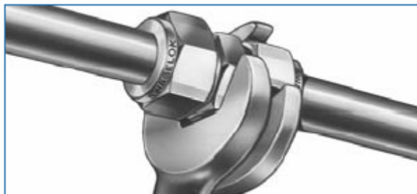
Figure 35: Insertion of the crimped tube into a coupling
