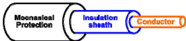
Figure 40: Construction of a 'standard' cable
