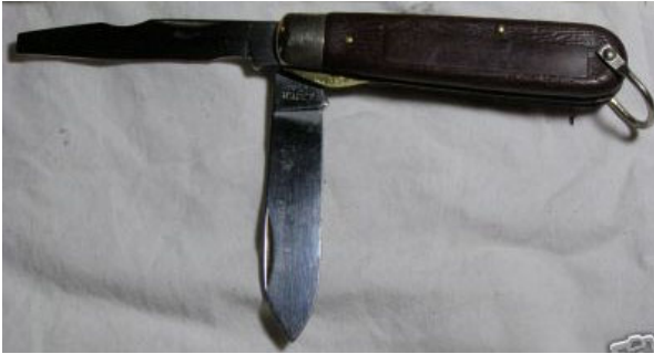
Figure 119: Typical electrician's stripping knife
