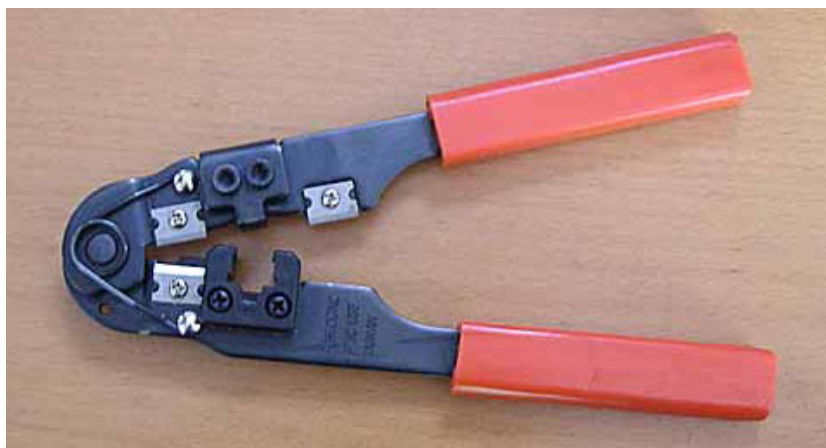
Figure 66: Crimping tool for RJ45 connectors (1)
