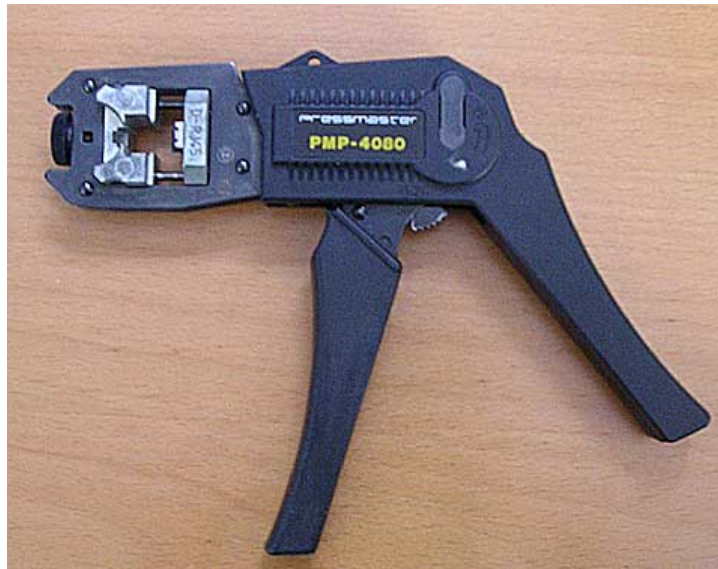
Figure 67: Crimping tool for RJ45 connectors (2)
