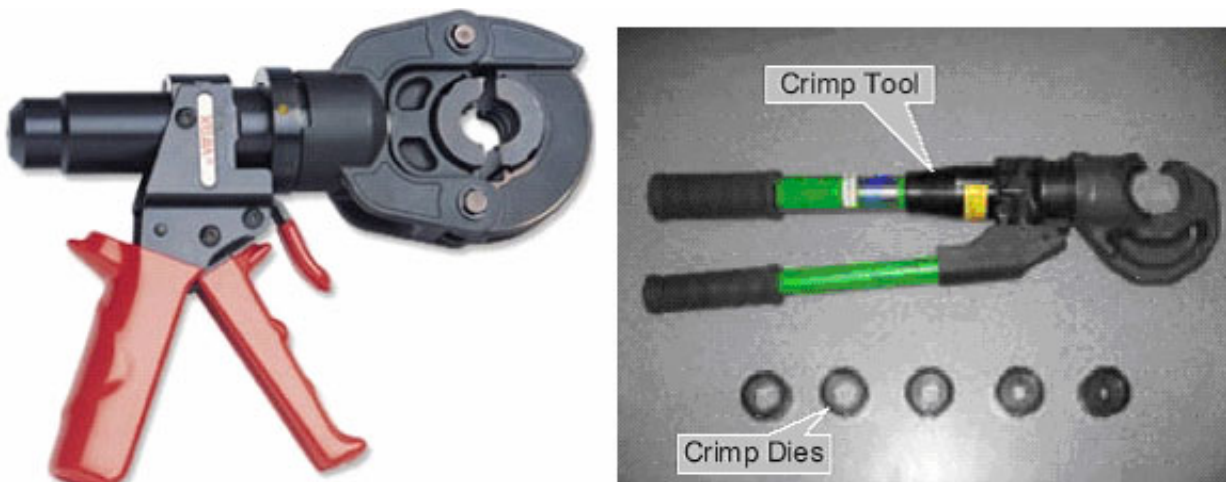
Figure 141: Hydraulic hand-operated crimping tool
