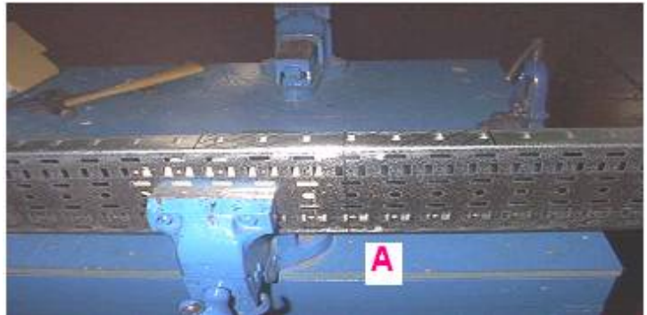
Figure 97: Construction of a flat 90° bend (A)
