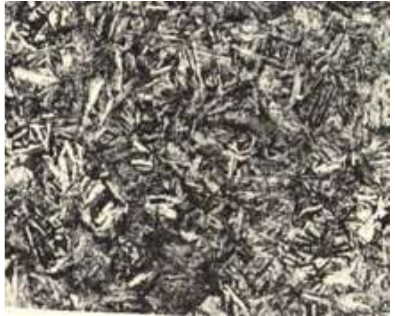
Bainite at high magnification
