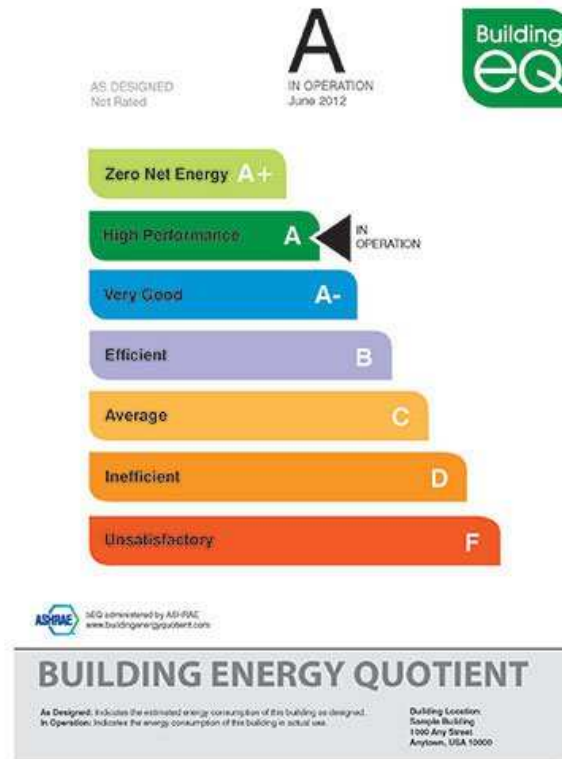
Figure 2-1 Sample Building EQ plaque.
