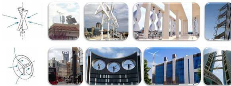
Figure 10-8 Examples of vertical (top row) and horizontal stand-alone (bottom row) and building-integrated wind turbines.
