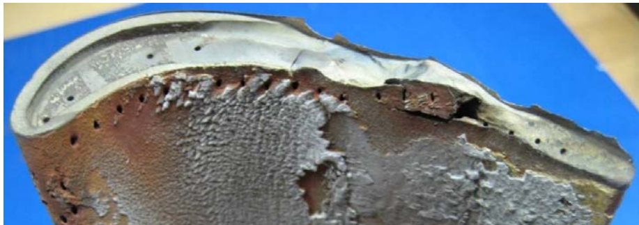
Repair Service B– Total tip replacement Using conventional weld alloy
