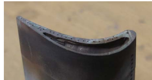
GE LM1600 Stage 1 Blade after 26,000 hours
