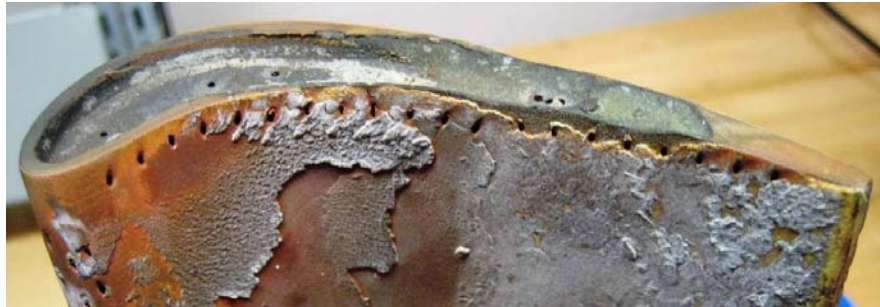
Repair Service A – Using conventional weld alloy
