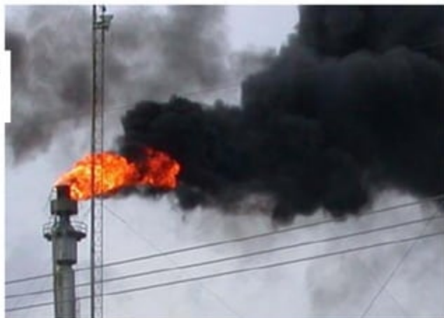
Ethylene steam flare without the steam
