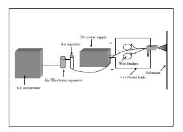
Figure 2-6. Typical two-wire arc spray system
