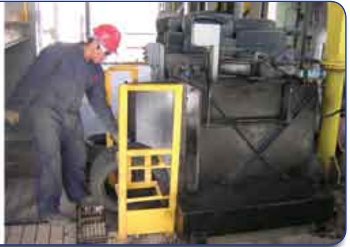
Exhibit 4-5. Tire metering systems for kiln introduction Photo courtesy of Terry Gray, TAG
