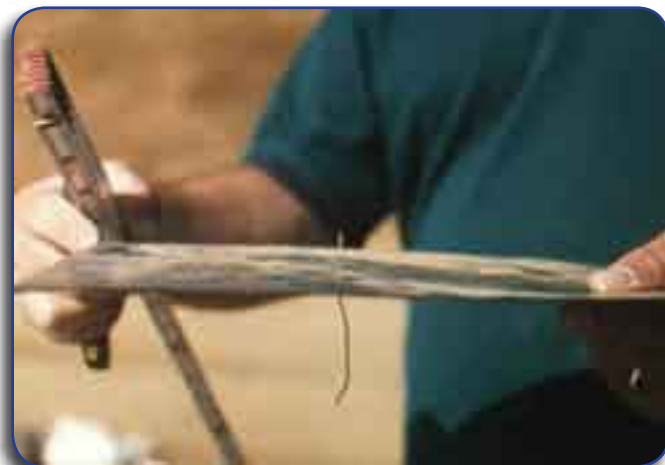
Exhibit 5-3. Example of steel bead wire puncturing geomembrane (Ref. 12)
