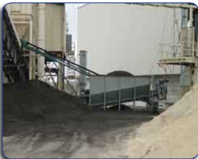
Metering system to introduce TDF into wood mixture before processing Photo courtesy of Terry Gray, TAG
