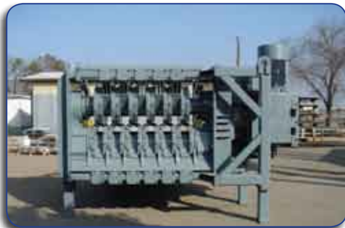
Exhibit 6-3. Tire shredder with 6-inch spaced knives Photo courtesy of Barclay Roto-Shred Inc., Stockton, CA
