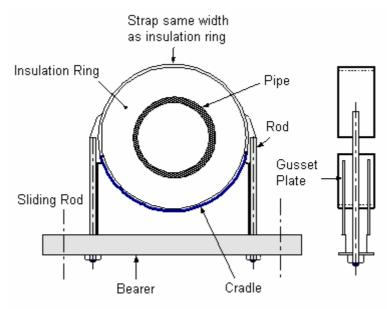
U - Bolt Cradle Using Insulation Ring
