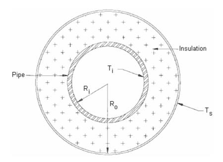
Cross-section of an insulated pipe
