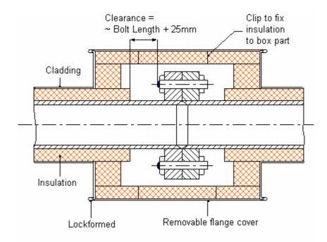
Typical Method of Insulating Pipe Flanges
