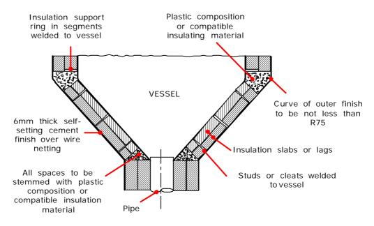
TYPICAL METHOD FOR INSULATING VESSELS WITH CONICAL BOTTOM
