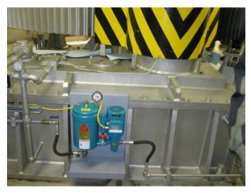
Figure 6-4. Kidney Filter for a Gearbox.
