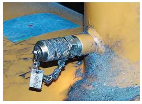
Figure 7-4. Minimess sample Valve.
