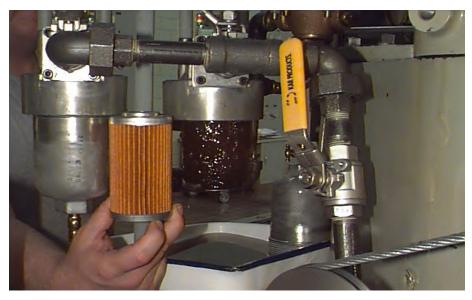
Figure 7-5. Varnish in a System That Resulted When ASTM D7155, "Oil Compatibility Testing," Was Not Performed.
