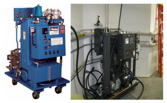
Figure 6-3. Vacuum Dehydrator.
