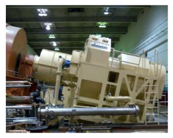
Figure 7-2. Gear Box (2:33,800 hp)
