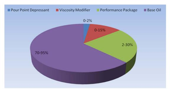
Figure 5-1. Typical Lubricant Composition.
