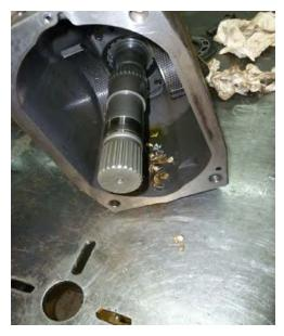
Figure 6-5. Cavitation Damage on a Hydraulic Pump.
