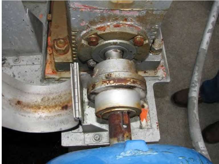
Figure 16-2. Gear Coupling with Grease Fitting.
