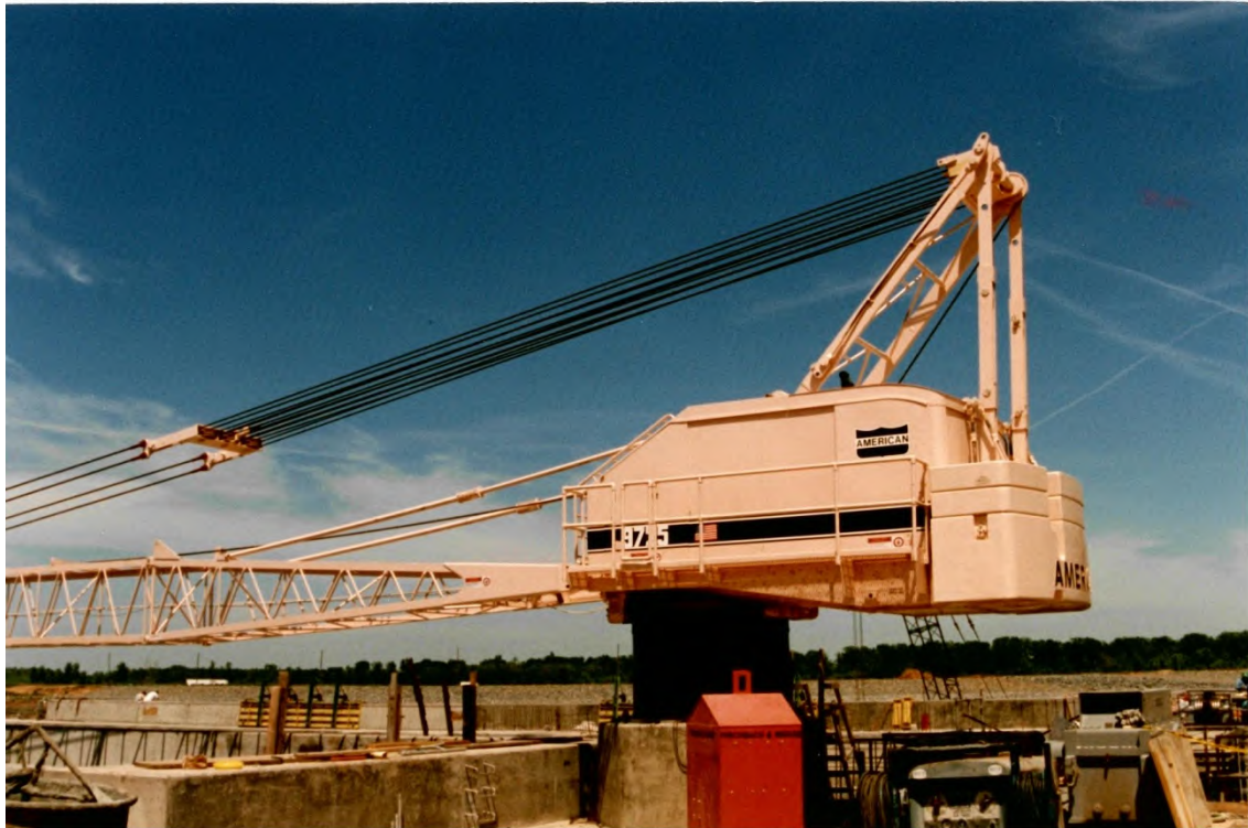
Figure 16-3. Pedestal Mounted Crane for Lifting Bulkheads.
