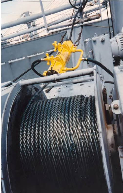
Figure 16-5. Wire Rope Lubricator.
