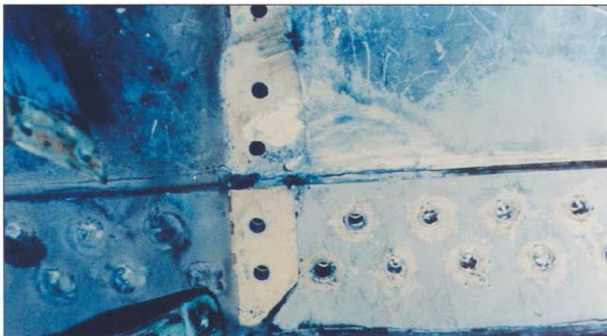
Figure 5-13. Corrosion Behind a Structural Component on a Wing Spar
