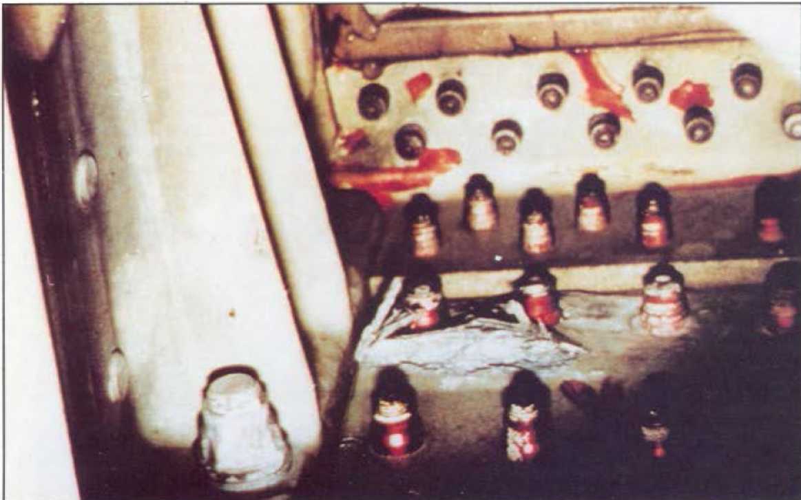
Figure 2-9. Severe Exfoliation Corrosion
