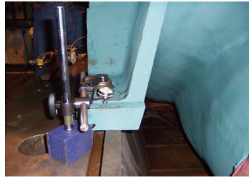
Figure 11. Pump Feet with Dial Indicator.
