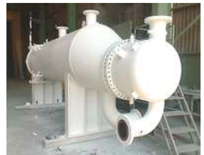
Heat Exchanger Final Painting Evaluation
