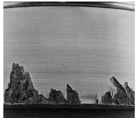
Geometric Stress Concentration (GSC) spalling.
