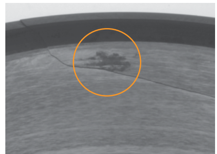
This ball bearing inner ring fracture resulted from installation on top of a metal contaminant or raised metal nick.
