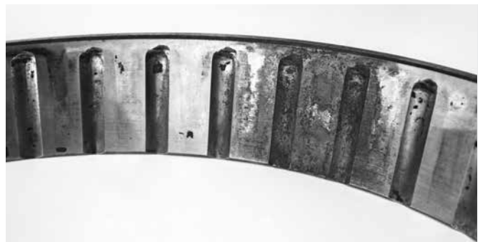
Heavy false brinell on outer race.
