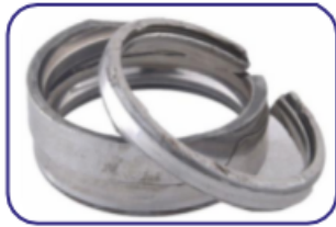
Fatigue fracture of Outerring caused by insufficient support in the housing
