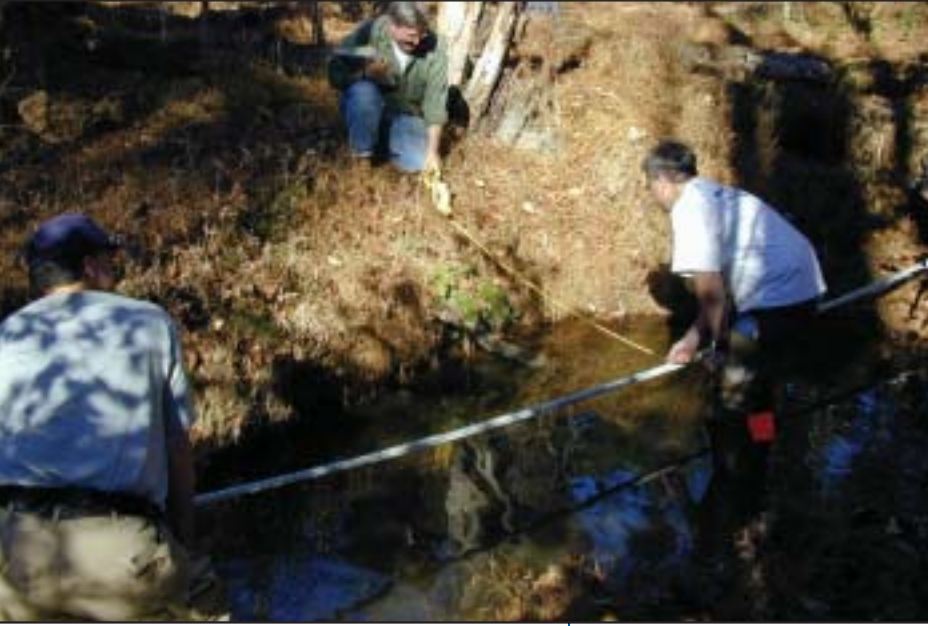
Figure 2.8 Field measurement of radius of curvature
