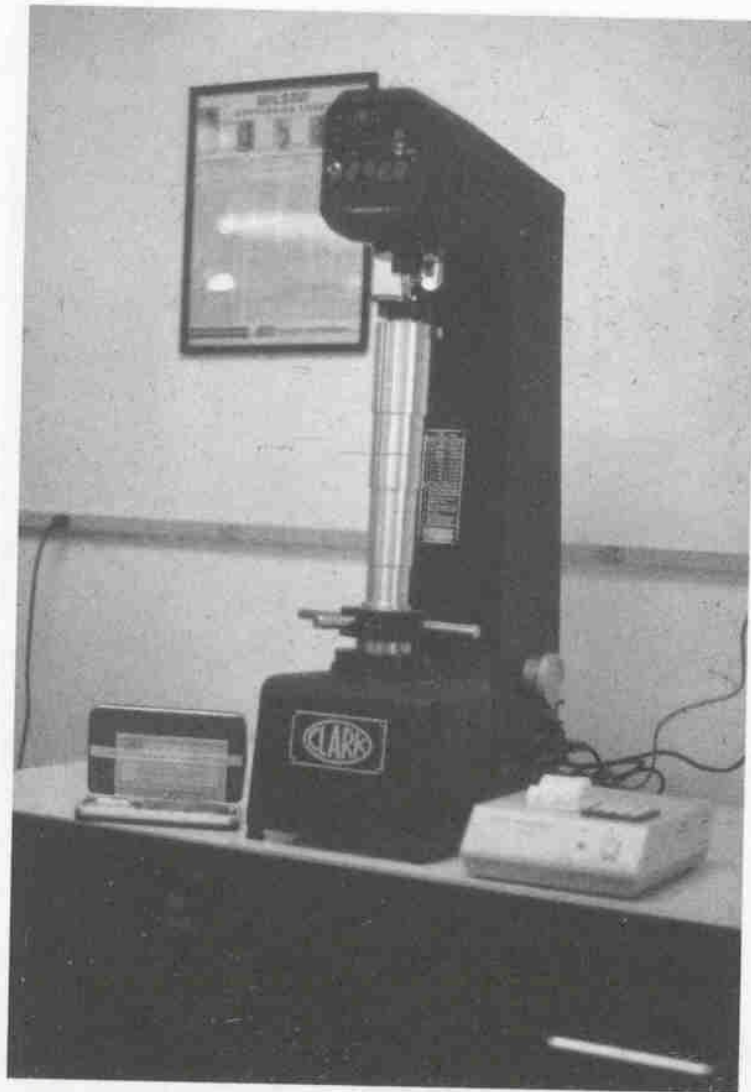
FIGURE 1-18 Typical hardness tester. (Courtesy of J. Devis Collection.)
