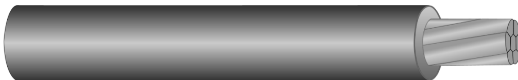
Figure 3.14: Example of a covered conductor construction
