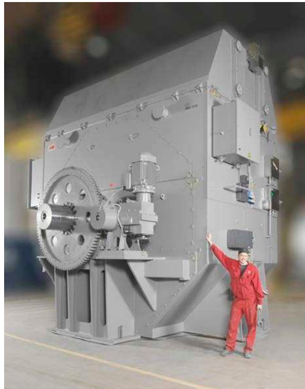
Figure 3.71: Reciprocating compressor motor 24 MW
