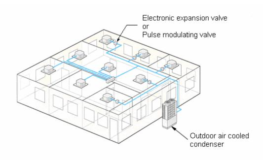
VRF System with Multiple Indoor Evaporator Units
