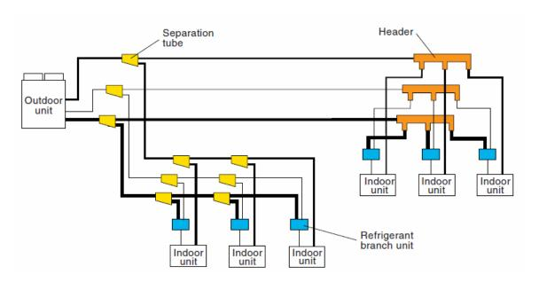
**Heat Recovery Type VRF System - Figure (Source: Fujitsu)**
