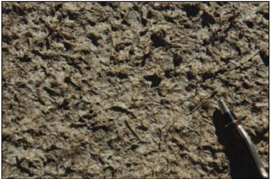
Figure 4—Hydromulch fibers form a smooth dense mat.
