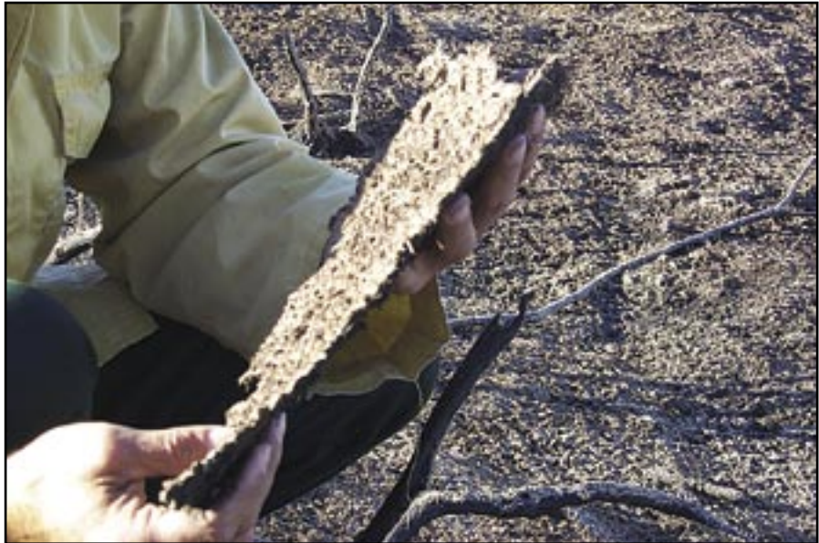
Figure 5—The relative thickness of the aerial hydromulch application.
