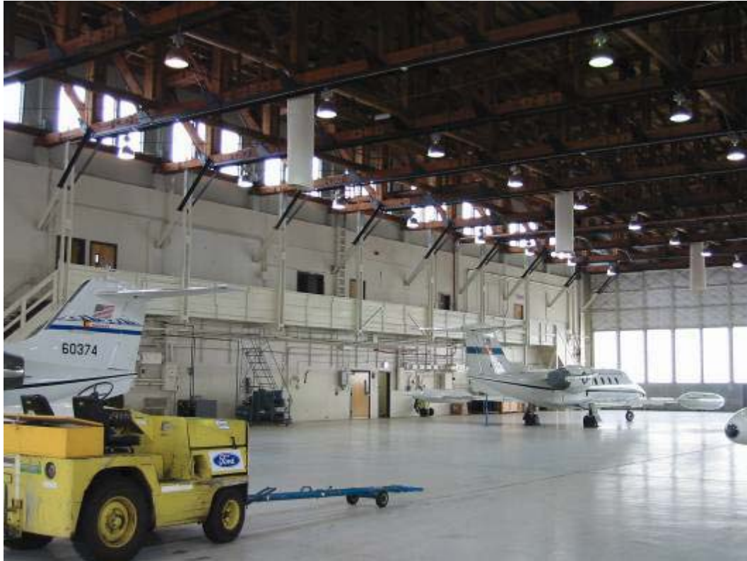
Figure 12 Example of Clerestory Application
