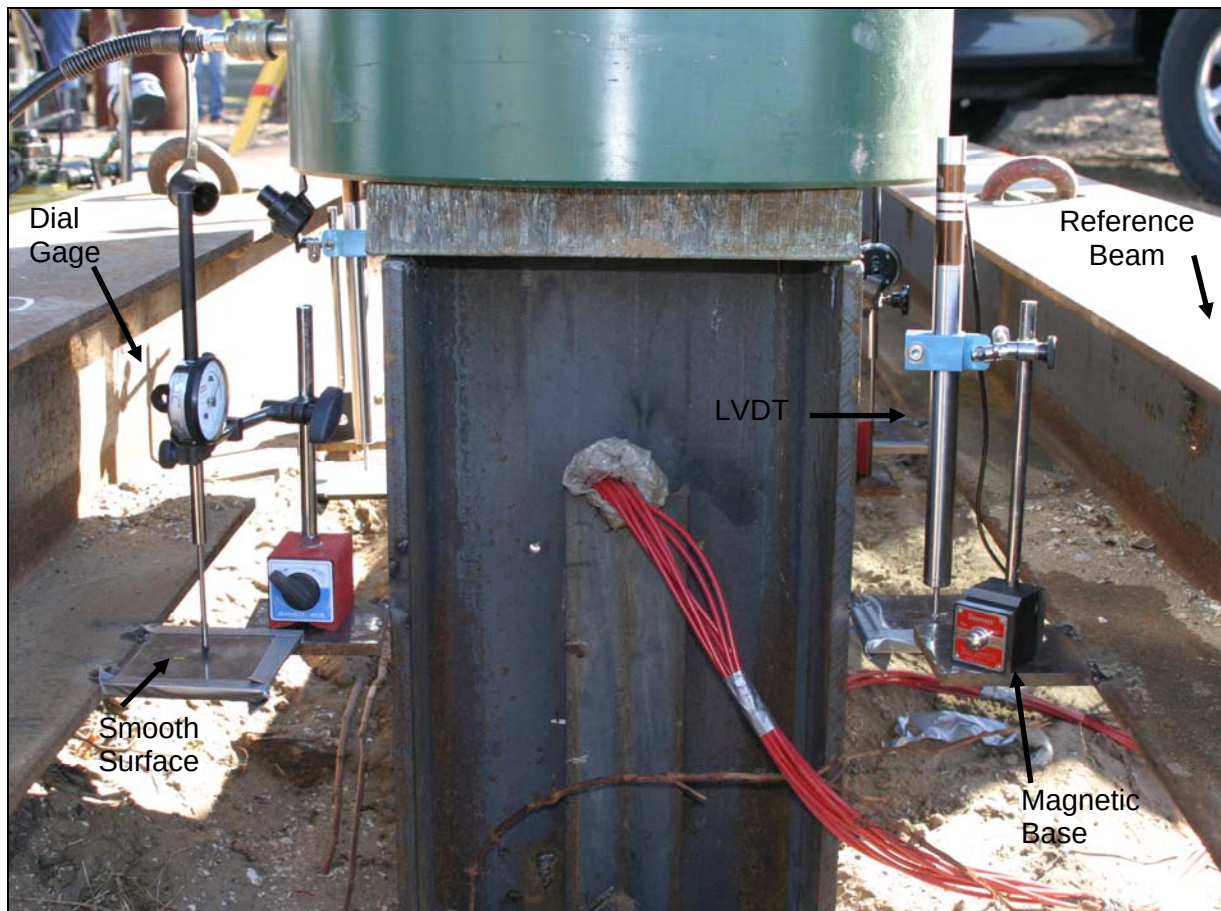
Figure 9-65. Load test movement monitoring components (FHWA, 2006a).
