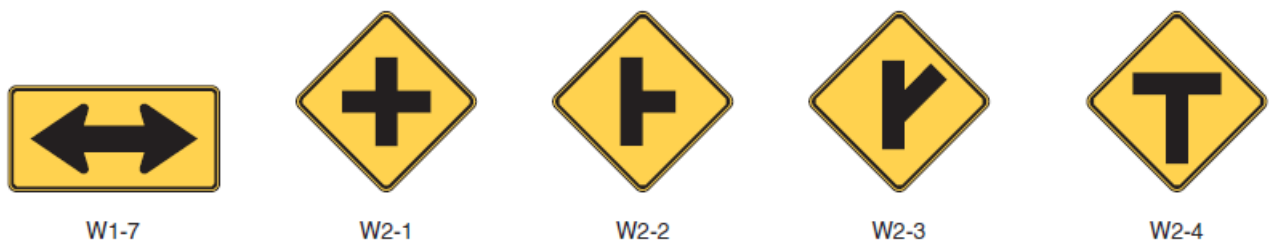
Figure 2C-9. Intersection Warning Signs and Plaques
