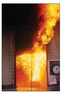
Figure 18–1. Flashover in standard room test.
