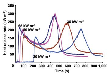
Figure 18–2. Heat release rate curves for 12-mm-thick oriented strandboard (OSB) exposed to constant heat flux of 20, 35, 50 and 65 kW m<sup>-2</sup>.
