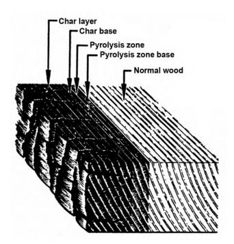
Figure 18-3. Illustration of charring of wood slab.
