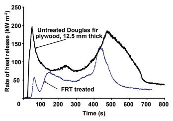
Figure 18–4. Heat release curves for untreated and fireretardant-treated (FRT) Douglas-fir plywood, 12.5 mm thick.
