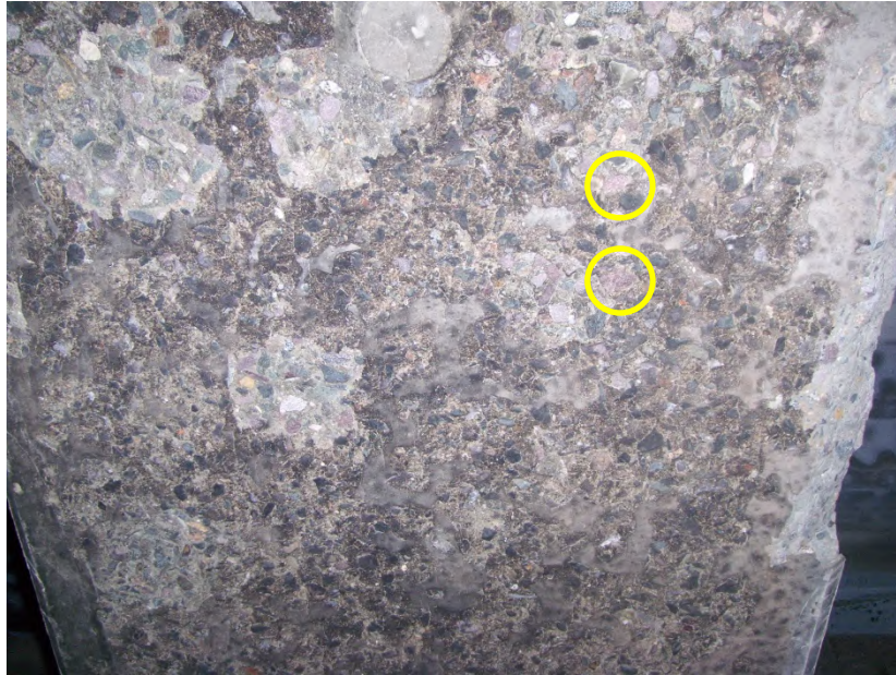
Figure 4.7 – Color change can indicate the highest temperature experienced.
