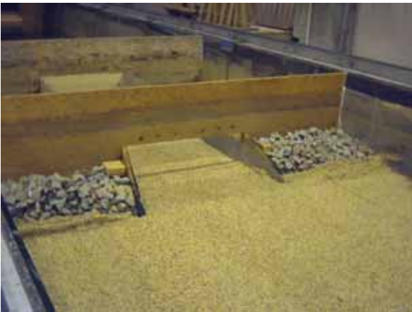
Figure 28. Photo. 8-degree inlet wingwalls before scour.
