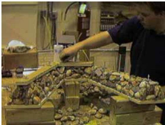
Figure 58. Photo. Fabrication of the cross vane.
