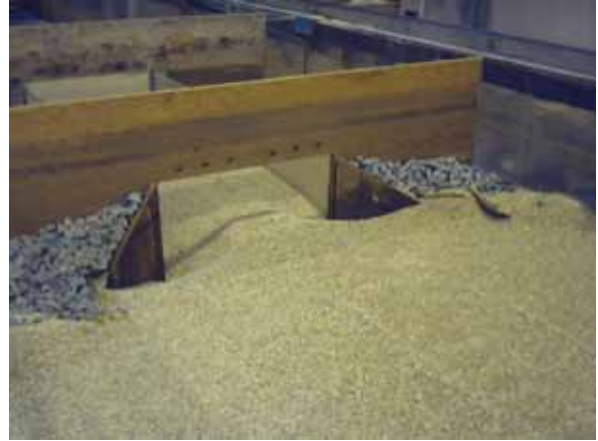
Figure 27. Photo. 45-degree inlet wingwalls after scour.
