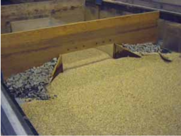
Figure 26. Photo. 45-degree inlet wingwalls before scour.
