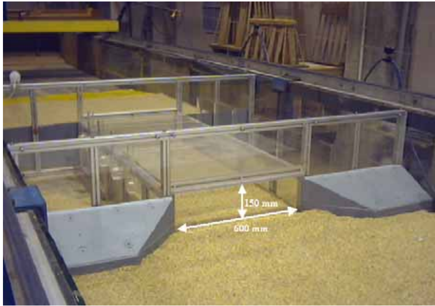
Figure 2. Photo. Rectangular culvert.
