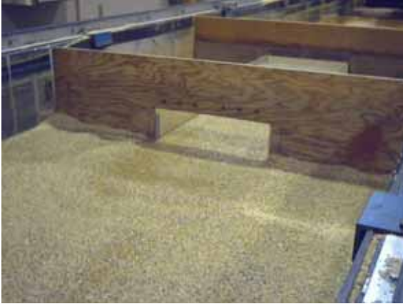
Figure 31. Photo. Truncated, circular wingwalls before scour.
