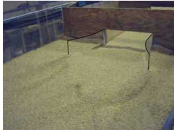
Figure 34. Photo. Elongated, streamlined wingwalls after scour.
