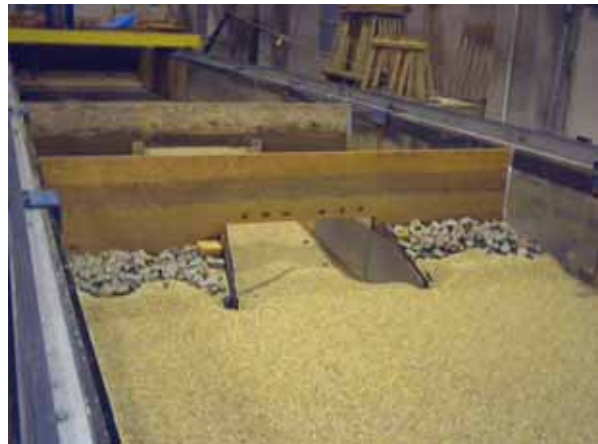
Figure 29. Photo. 8-degree inlet wingwalls after scour.
