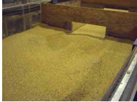
Figure 32. Photo. Truncated, circular wingwalls after scour.
