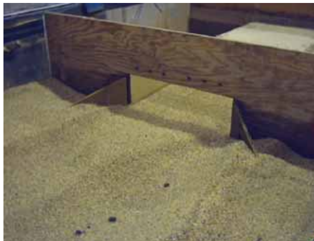
Figure 40. Photo. 45-degree wingwalls after scour.
